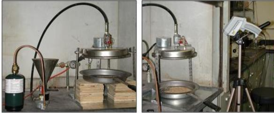
Figure 1:3. Bench top model of infrared emitter (left) showing the propane bottle and pan with hard red winter wheat. The non-contact thermometer (Raytek®, Model MX4) is used for continuous measurement of temperatures attained by wheat (right) during exposure to infrared via a RS-232 cable connected to a laptop computer. Photos by Bh. Subramanyam.
