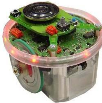
Figure 2-1 E-puck Mobile Robot
