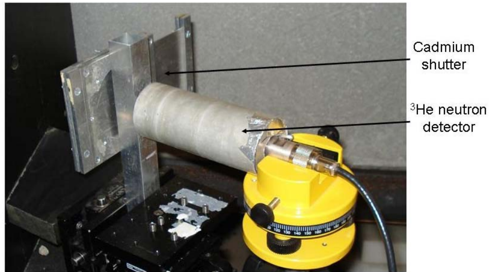
Figure 4.30: ^3\text{He} detector used to determine the neutron intensity at the test port opening.
