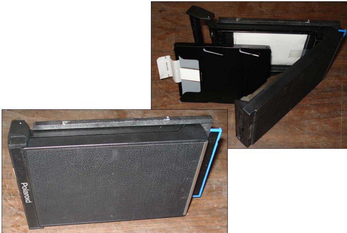
Figure 4.29: Polaroid film cassette (left) with NE426 (white sheet inside) installed (right) used to measure the uniformity of the diffracted neutron beam at the test port.
