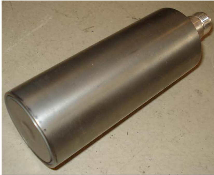
Figure 4.5: Reuter Stokes ^3\text{He} neutron detector.
