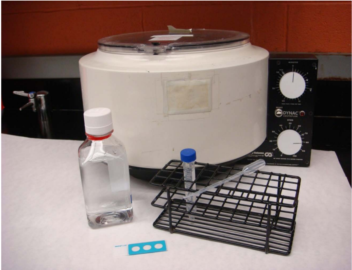
Figure A.6 Materials needed to perform the MeriFluor® Cryptosporidium / Giardia direct immunofluorescent assay; a fixed head centrifuge, PBS-EDTA solution, 15 ml conical centrifuge tube, and MeriFluor® Cryptosporidium / Giardia direct immunofluorescent assay microscope slide (rest of test kit not shown).
