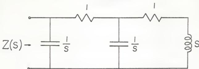
This driving point impedance will act as a pulse stretcher and will reduce the magnitude of the input spike voltage at the load impedance  $(1 + s)$ .
