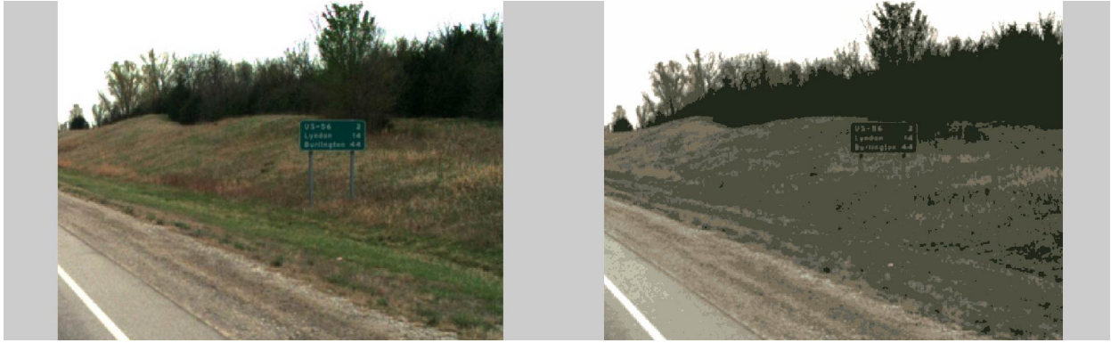
Figure 2.2: Here, the green sign's color is not one of the 16 color centers. Its pixels are shifted to the closest cluster center resulting in under segmentation.
