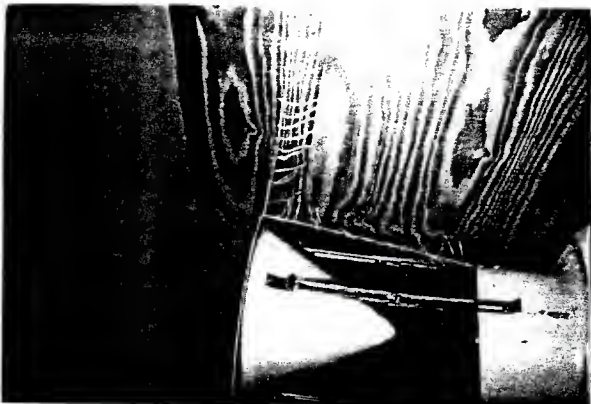
Figure 44. Interaction between a 8 mps wind and fan airflow with the 60° wind diverter
