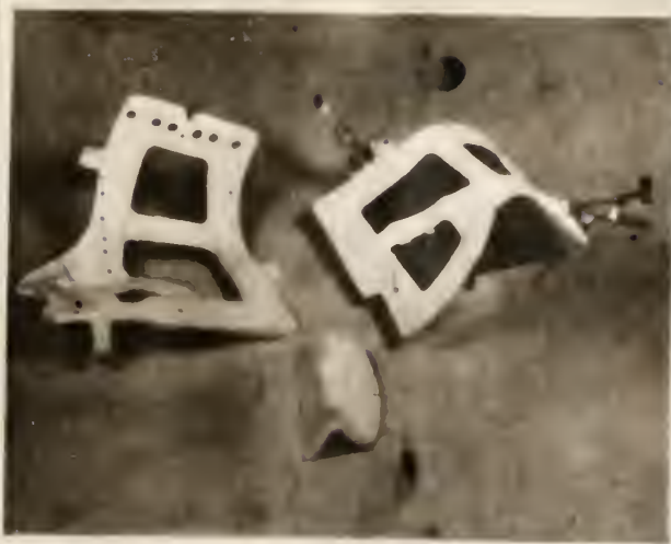
Aircraft drill jig and scribe template.
