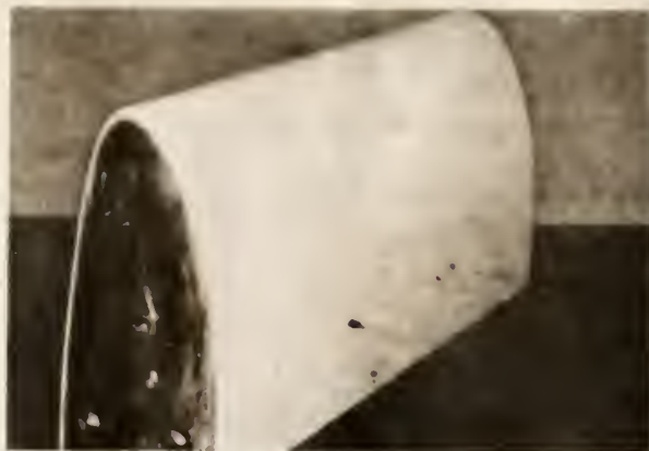
Aircraft form blocks for inter-wing de-icer skins. The surface cast on kirksite cors.
