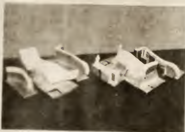
Aluminum cast frames, surface cast with plastic material. Tools used for checking fixtures.
