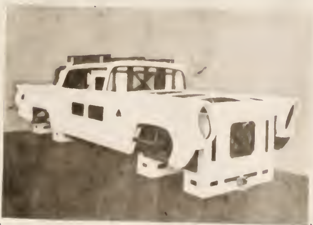
Laminated plastic body stack for an automobile. All the body sections are fitted to a master cube. The frame structure of the cube and each body section is made of plastic tubing.
