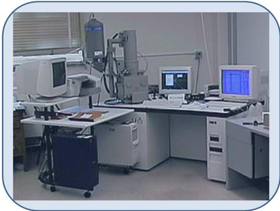
Fig. 2.3 Photograph of SEM interfaced with NPGS (for e-beam lithography) and EDX (for composition determination) system located in our lab.
