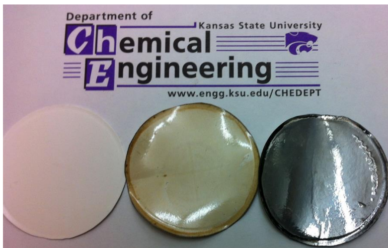
Figure 4.4 – PEI membranes that are: (left) virgin, (middle) coated with \text{RuCl}_3 , and (right) coated and reduced.
