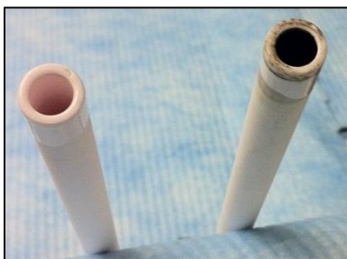
Figure 2.4 - Virgin membrane (left side) and catalytic membrane (right side). The darker color on the bore side of the membrane on the right indicates that PVP-Pd catalyst adhered to the selective layer.
