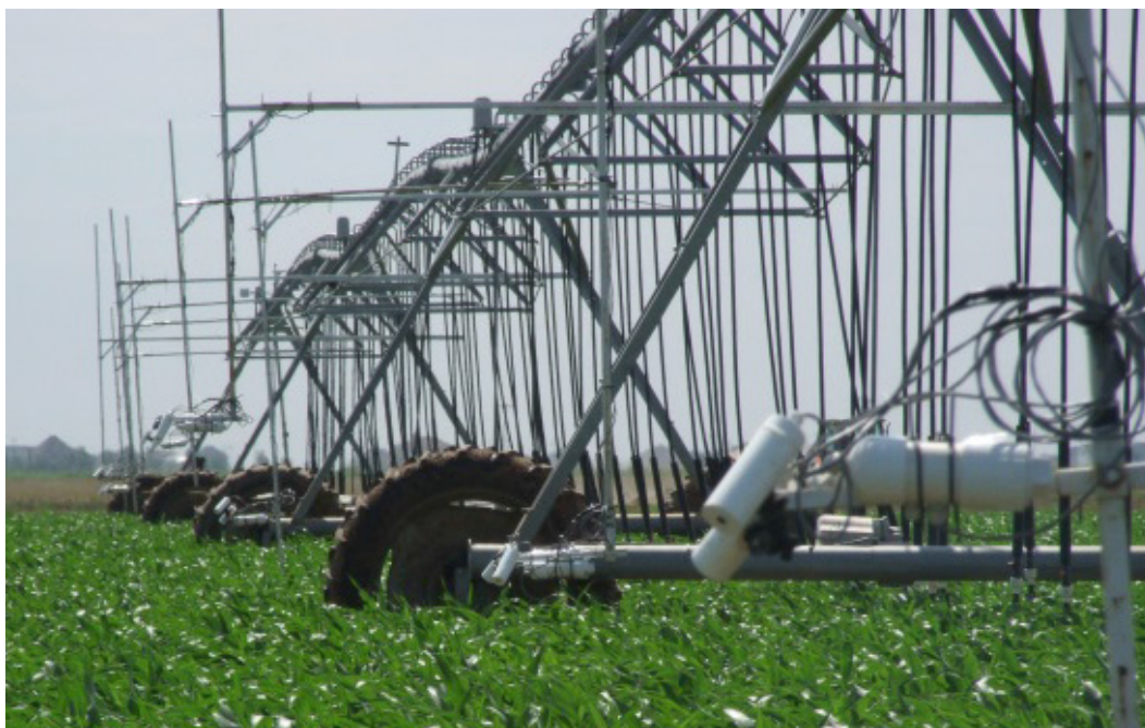
Figure 2. Canopy temperature sensors installed on a center pivot to automate irrigation scheduling of grain sorghum at USDA ARS, Bushland, TX (O’Shaughnessy et al., 2013).
