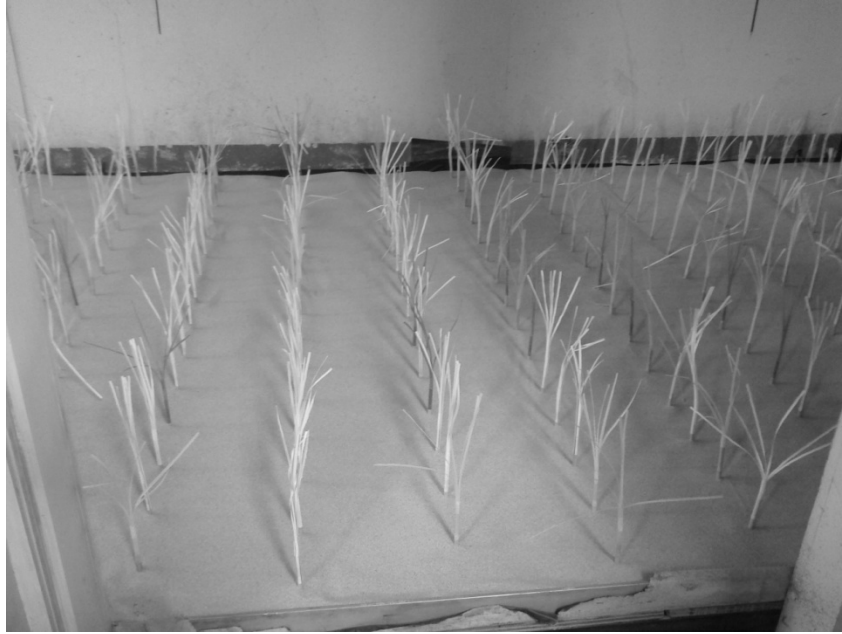
Figure 3.2. Dowel rods with plastic straws split 80 mm from the top to simulate young plants.
