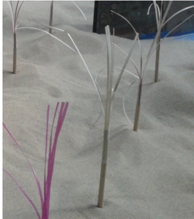
Figure 6.2. Actual standing vegetation model used in the wind tunnel.
