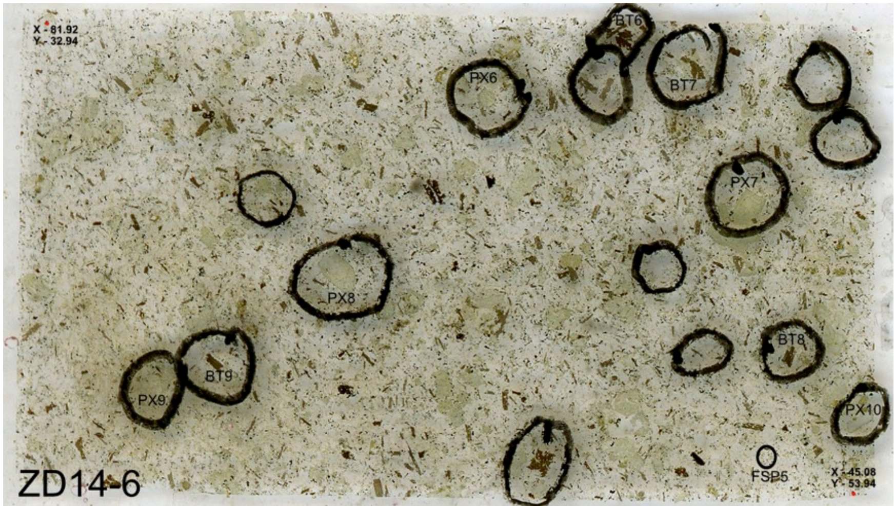
Figure C 5-2 Electronic scan of ZD14-6 thin section indication analyzed crystal locations.
