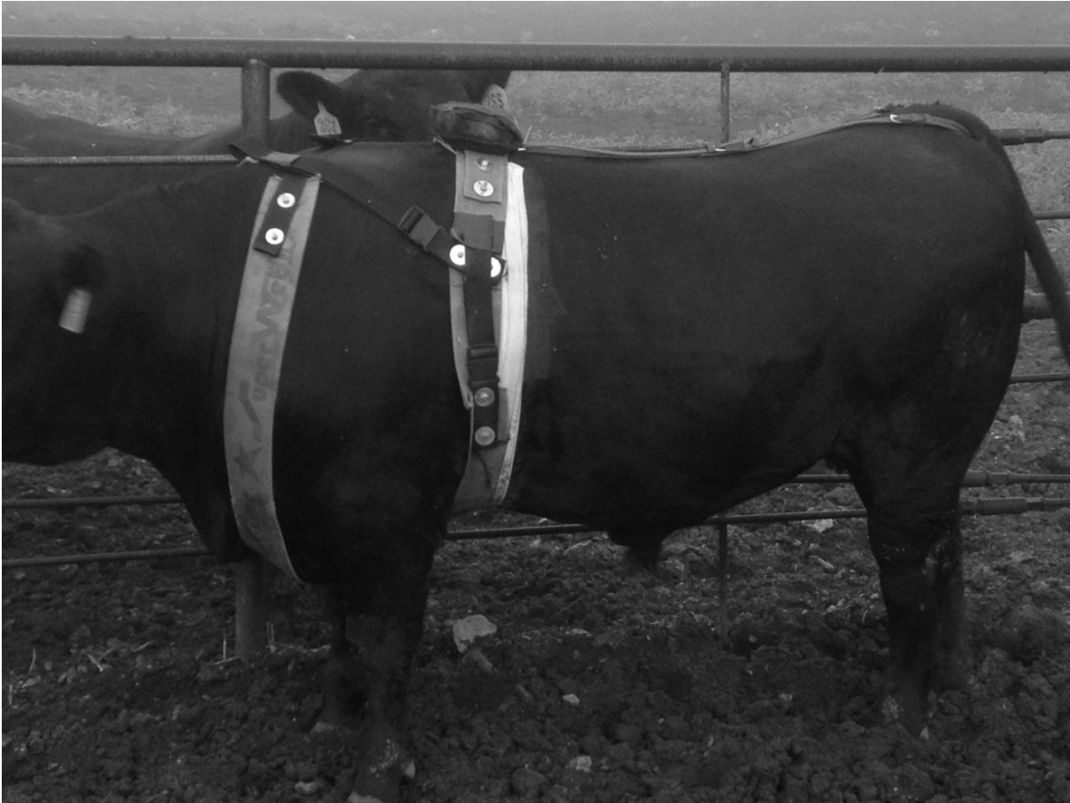
Figure 3-2 Illustration of Applied Holter Monitor and Harness.
