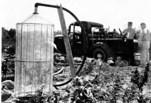
The transparent transpiration "hood" and other apparatus in operation at the nursery at the Hays Branch Experiment Station. This equipment measures the amount of water lost by a tree.
