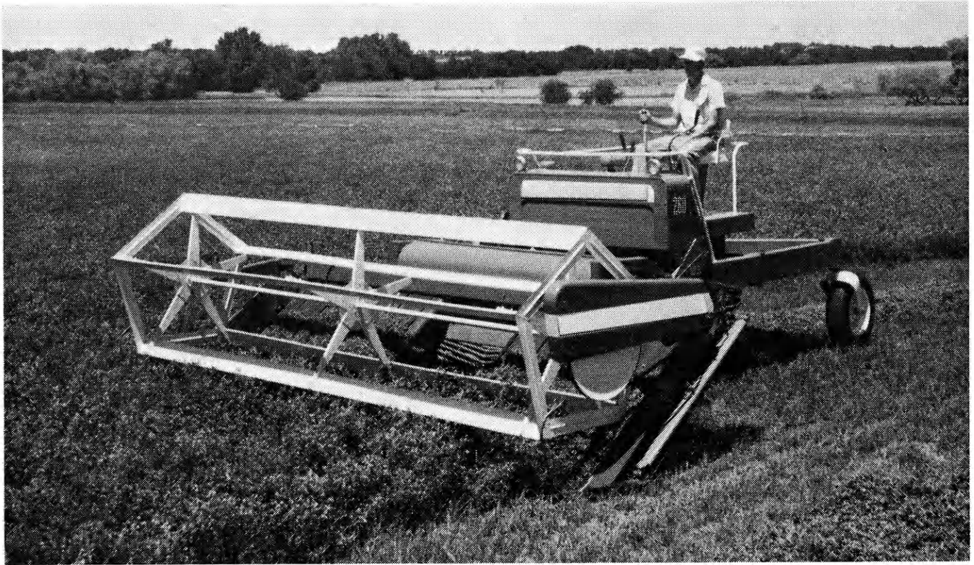
This self-propelled swather-windrower, equipped with a crimper-crusher conditioning attachment, has a capacity of 4.5 acres per hour.
