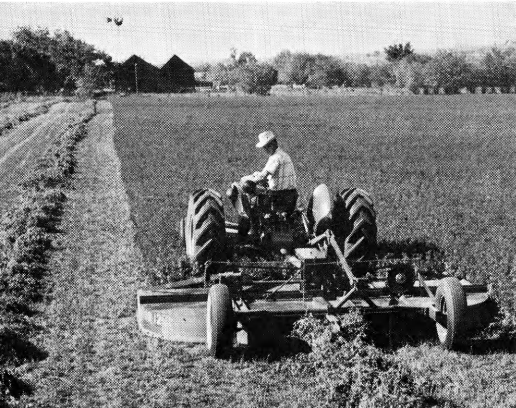
This 12-foot rotary mower cuts, lacerates and windrows hay—all in one field operation.
