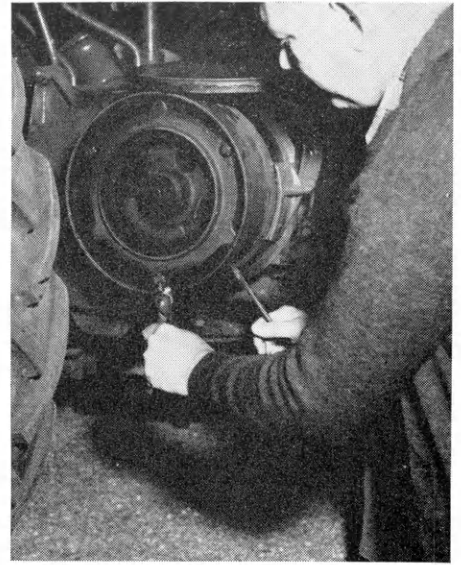
Cliff Hinkle, of the Standard Oil company, shows how to adjust a clutch pulley.
