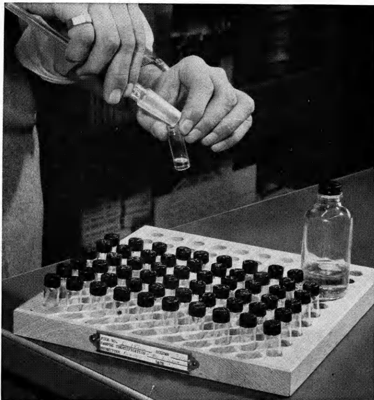
A laboratory assistant (above) takes a fraction from one of the new miniature stills at Standard Oil's Whiting laboratories. The small charge in the large bottle (below) can be separated into 60 fractions in these exact stills.
