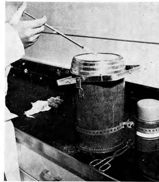
A KIT CARRIED by field men to keep semen frozen. The large thermos jar is filled with alcohol and dry ice. The small attached bottle contains cool alcohol for thawing.
