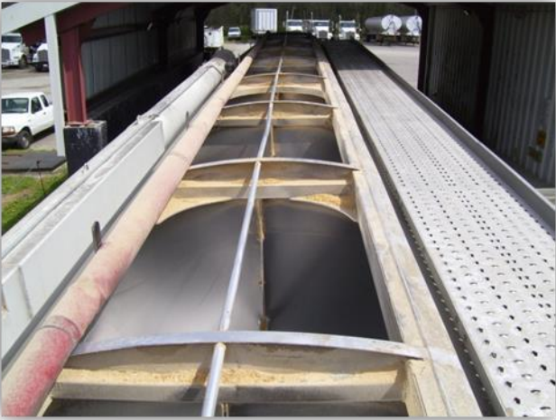
Figure 1.7 Potential contamination from left over material in the top of a bulk feed truck
