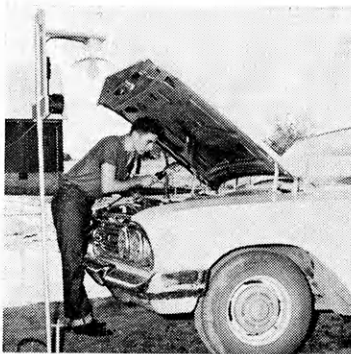
The portable lamp provides good area lighting and the "trouble" lamp provides light for "hard to get at" jobs.
