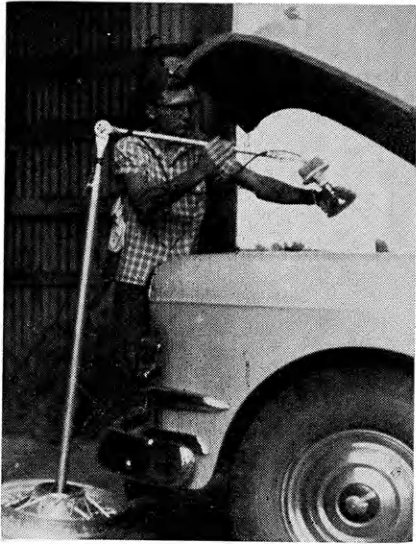
John Ryman of the Slate Creek Strivers Club, Sumner county, uses the shop lamp he made in the electric project. It has two knuckle adjustments and extends upright to 144 inches for an emergency yard light.
