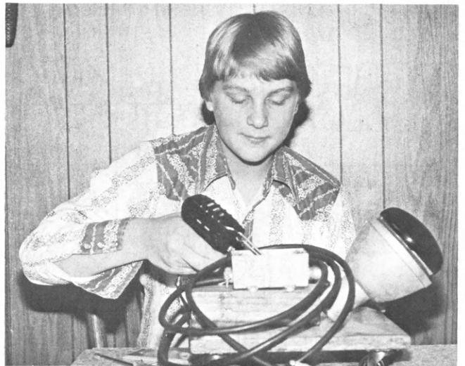
The Reno County 4-H member solders the switch box on the heat lamp he made his second year in the electric project.
