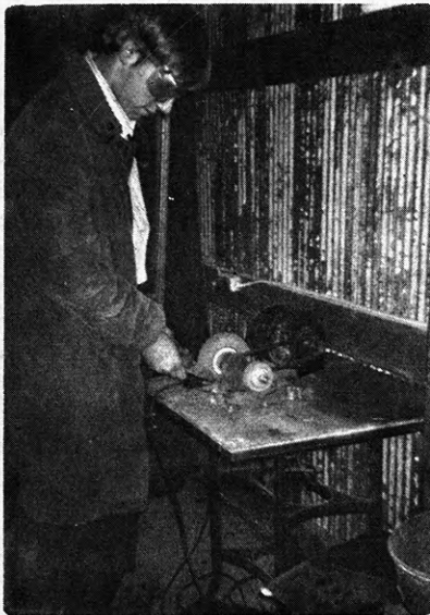
On the grinder he made, Dale sharpens a mower blade. The Sevarts mow lawns so the grinder was especially helpful in keeping lawnmower blades sharp.
