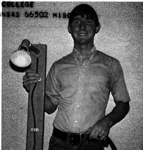
"This portable lamp went to state fair also. It hangs up and also has an outlet and switch box. It serves our needs much better at times than the portable outdoor lamp."
