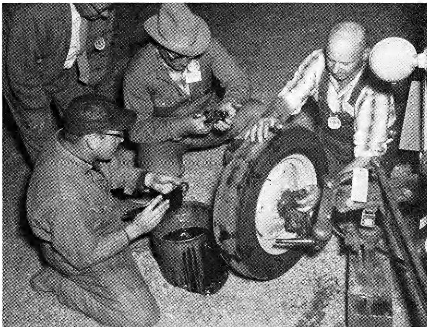
Packing front wheel bearings at the Hutchinson tractor leaders' clinic sponsored by Standard Oil are Bill VanSlike, Barton county club agent; Wilbur Cox, K. C. Tractor and Imp. Co.; Ray Beesley, Gove county; and Roy Stevens, Geary.
