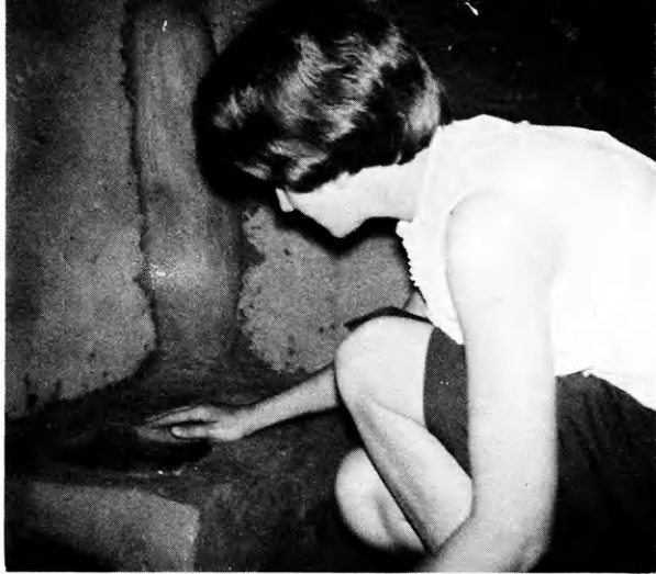
Mary K. Munson, IFYE to India, works on a Smokeless Chula in a village housewife's kitchen. It is made of mud and a big improvement over what had been used because the smoke is carried outside and the heat is more confined to the cooking area.
