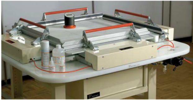
A skilled miller needs to identify the direction of the weave before stretching the cloth across the sieve for the appropriate sieving result. Photo courtesy of Sefar.
