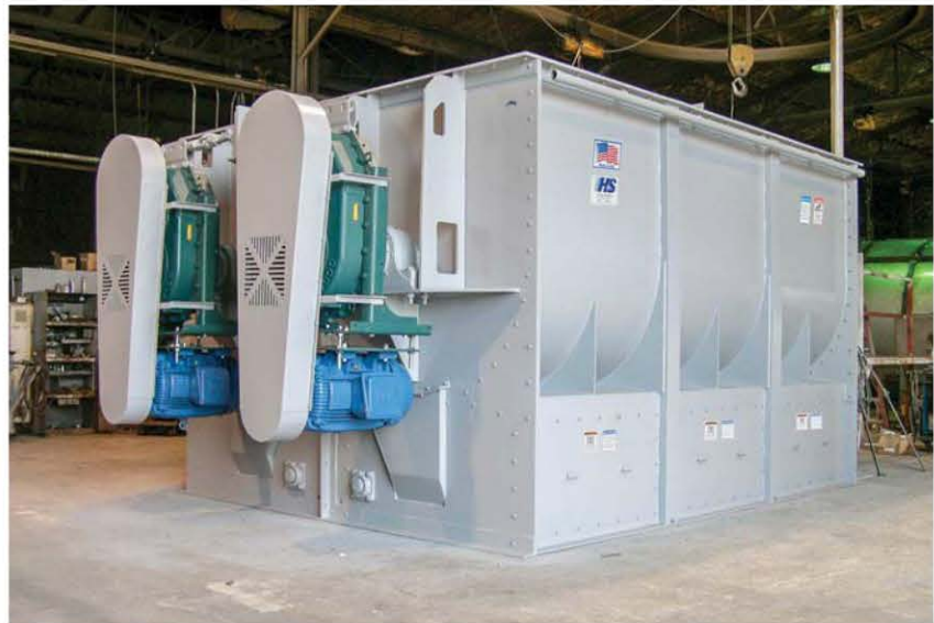
A twin shaft mixer manufactured by Hayes & Stolz. Photo courtesy of Hayes & Stolz.
