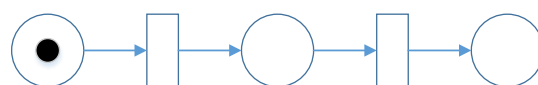
Figure 3.1- A very basic Petri net with three places (circles) and two transitions (rectangles)
