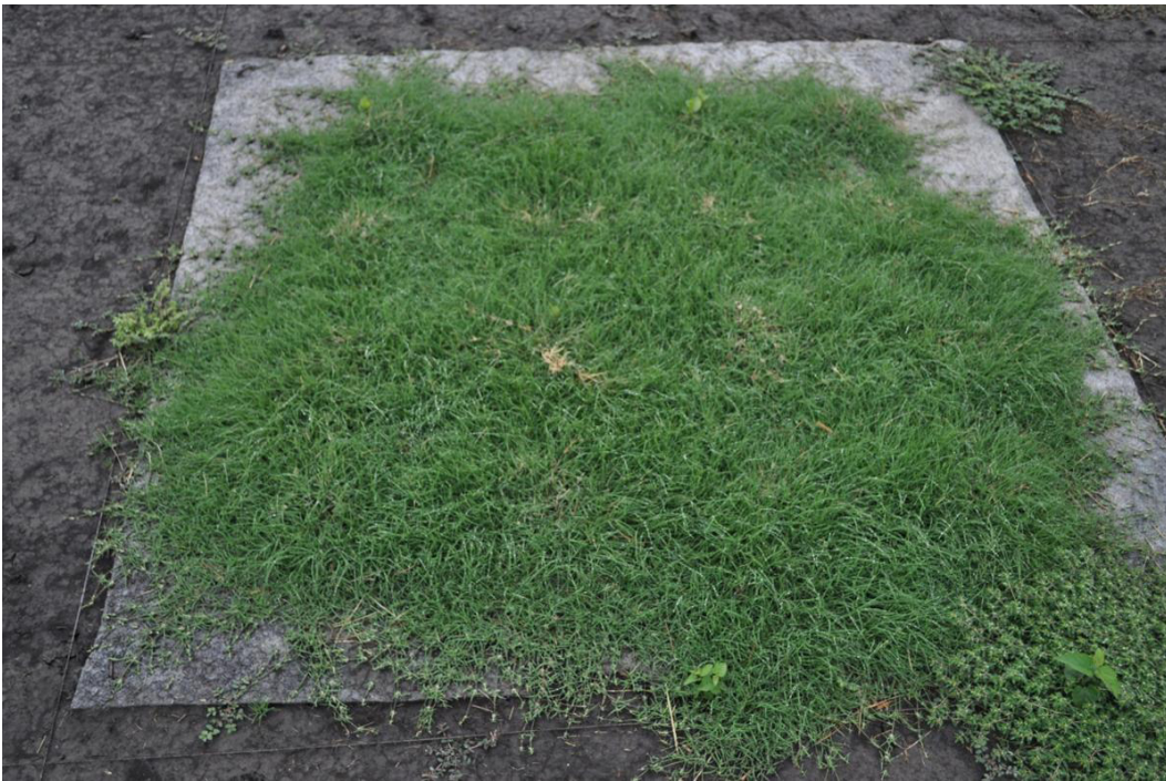
Figure 5. ‘Legacy’ buffalograss successfully established on a turf reinforcement mat.
