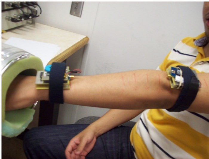
Figure 5.2 Transmitter and receiver are mounted directly on arm with initial distance of 30 cm before the arm is inserted inside the tube.
