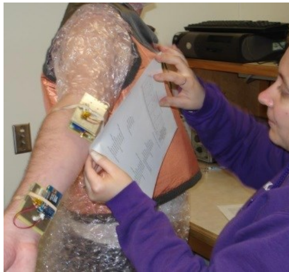
Figure 5.14 Transmitter and receiver placement
