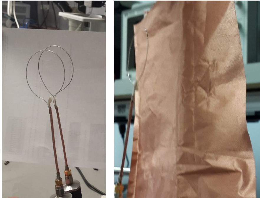
Figure 3.11 Measurement setup for Case 1 (without fabric) and Case 2 (with fabric): two small loop antennas separated by 3 cm
