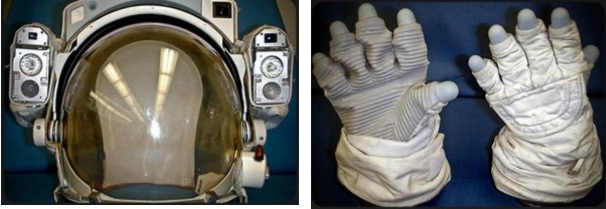
Figure 5.6 EMU space suit helmet (left) and EVA gloves (right) [91]
