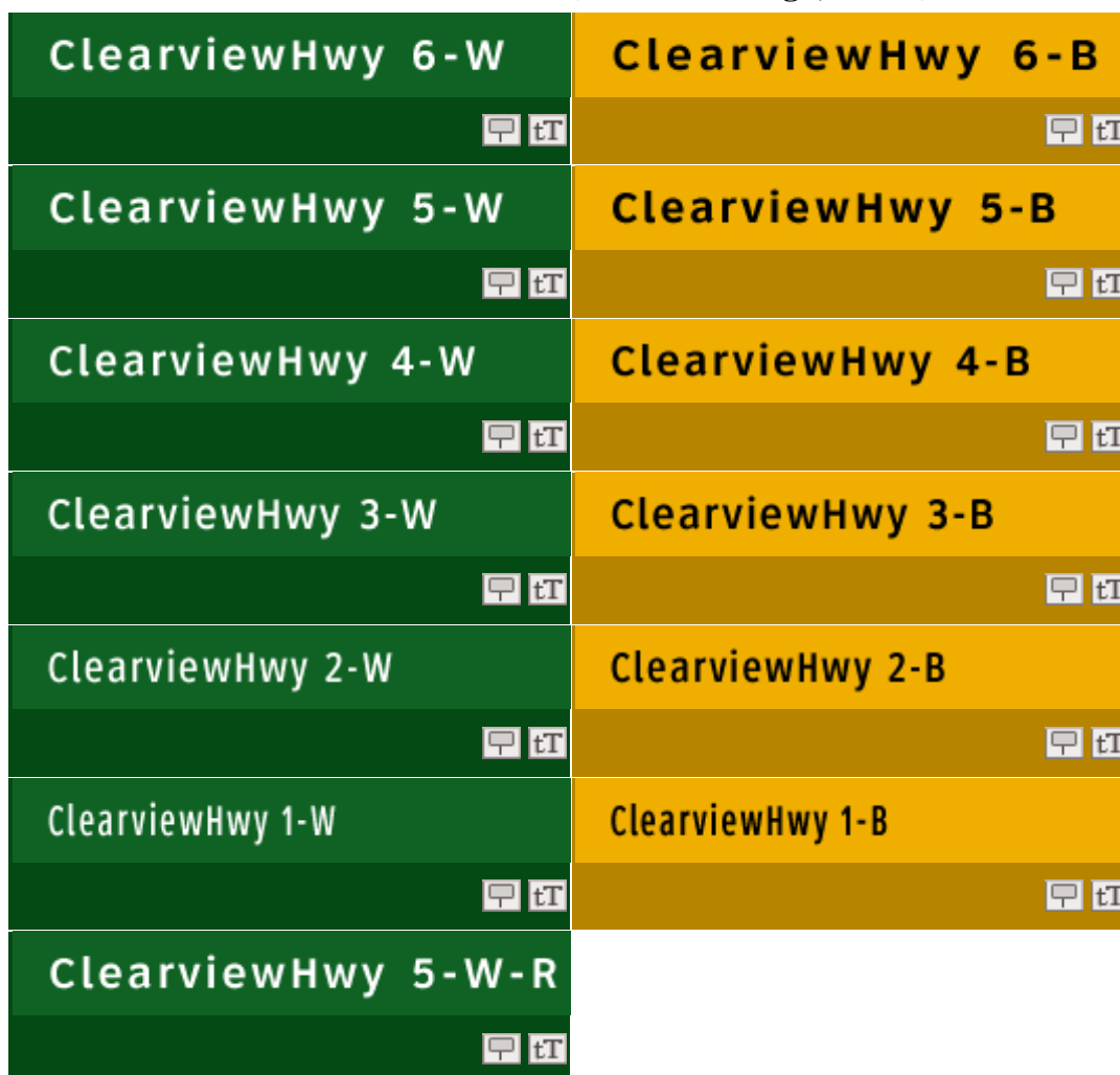
Figure 2.7 The Clearview Font Distinct Weights. Right Side Is Negative Contrast and Left Side Is Positive Contrast (Terminal Design, 2004b)
