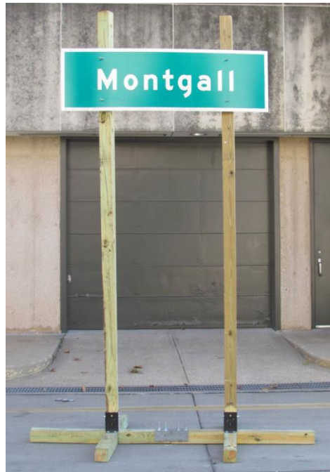
Figure 6.5 Post Used in the Experiment with One Mounted Sign
