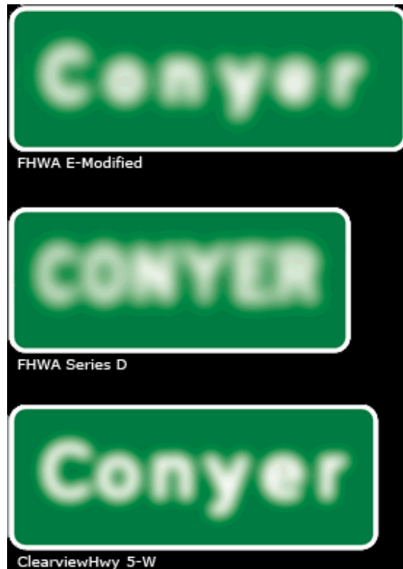
Figure 2.6 Irradiation or Halation Phenomenon for Three Font Styles (Terminal Design, 2004c)
