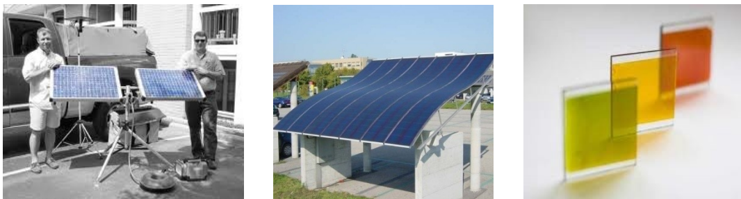
Figure 1.1 Images of three generations of solar cells. (left) the first generation solar cell, (middle) the second generation solar cell, (right) the third generation solar cell.
