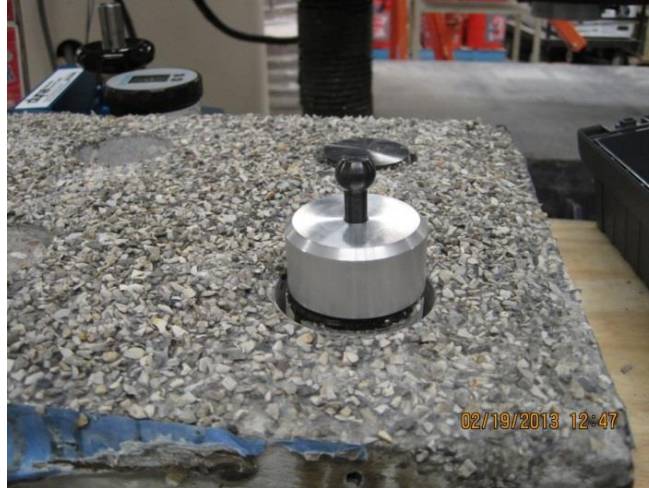
Figure 29: Pull-off cap ready to be tested
