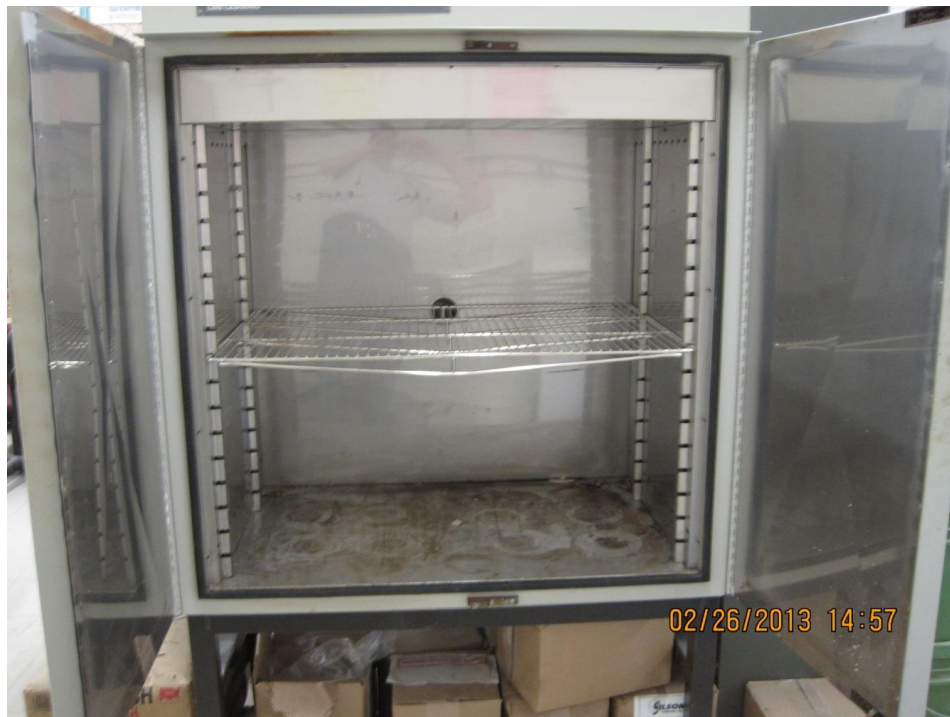
Figure 10: Wet cure location for 100F oven
