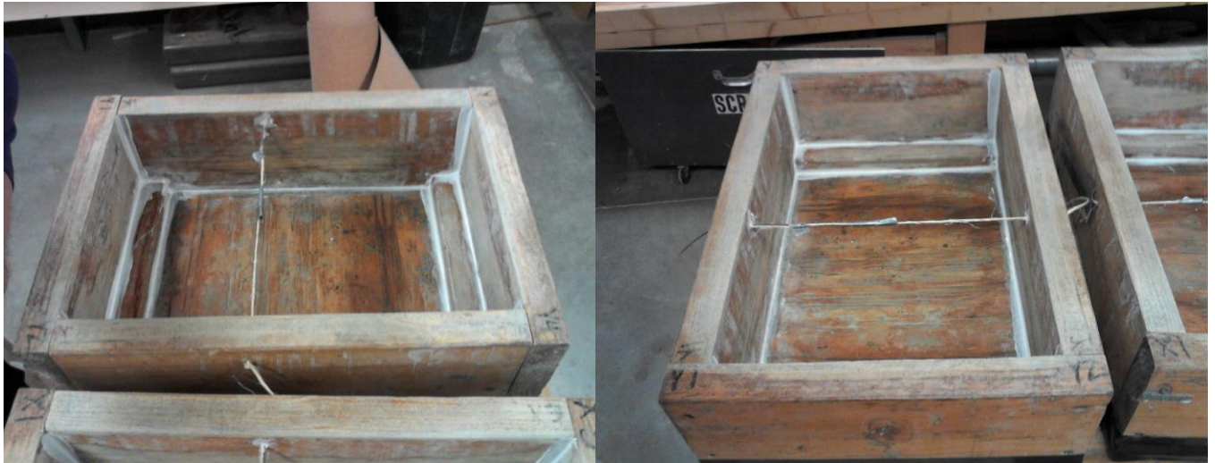
Figure 5: Forms built to accommodate the 12 x 18 x 6 inch slabs.
