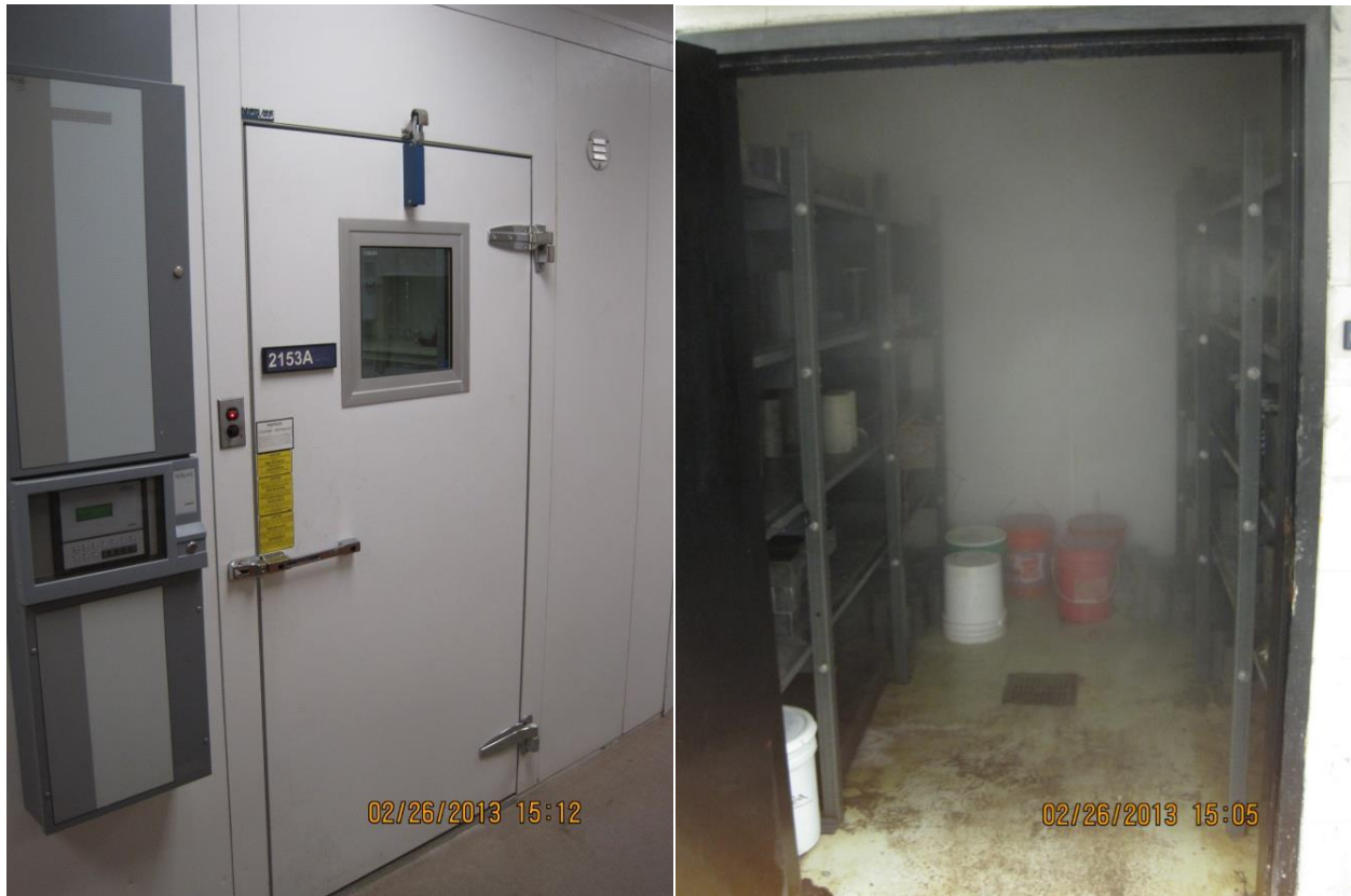
Figure 9: Wet cure locations for 40°F refrigerator (left) and 73°F moist room (right)
