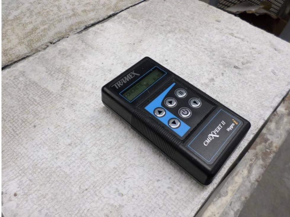
Figure 19: Tramex CMEXpert II instrument used to take moisture readings
