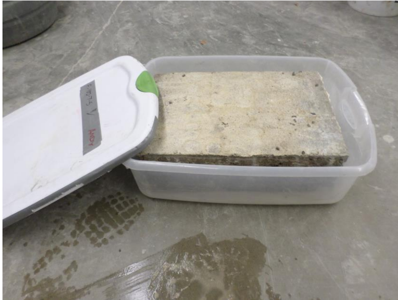
Figure 11: Slab placed inside a bin for wet curing
