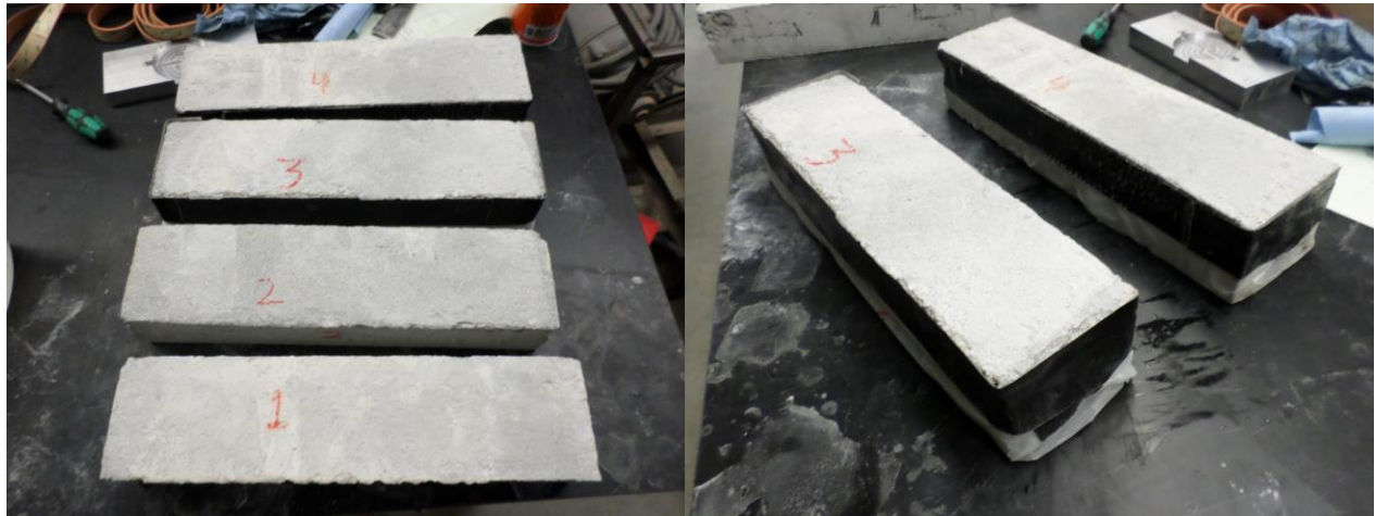
Figure 55: Test specimen cast to test moisture content
