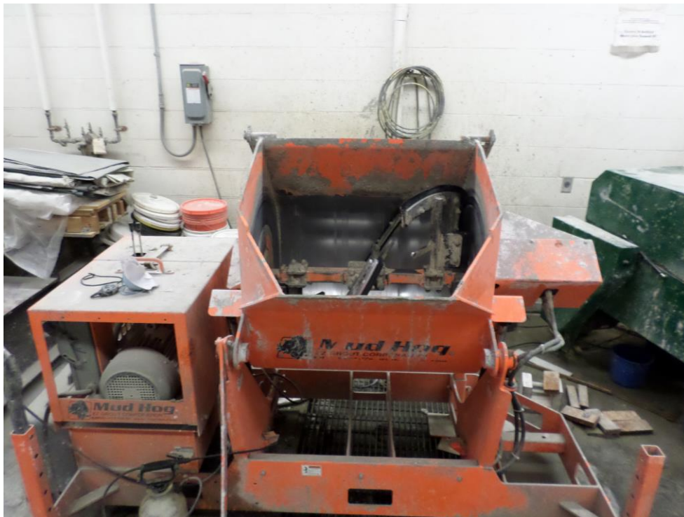
Figure 7: Mud Hog mixer used to batch concrete.
