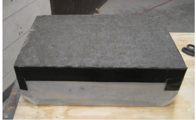
Figure 13: Slab wrapped in plastic to dry
