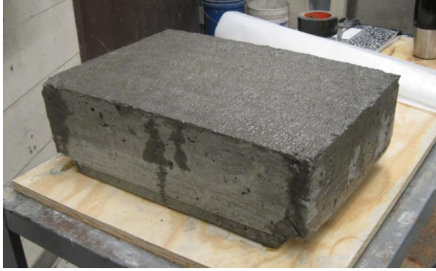
Figure 12: Slab after wet curing
