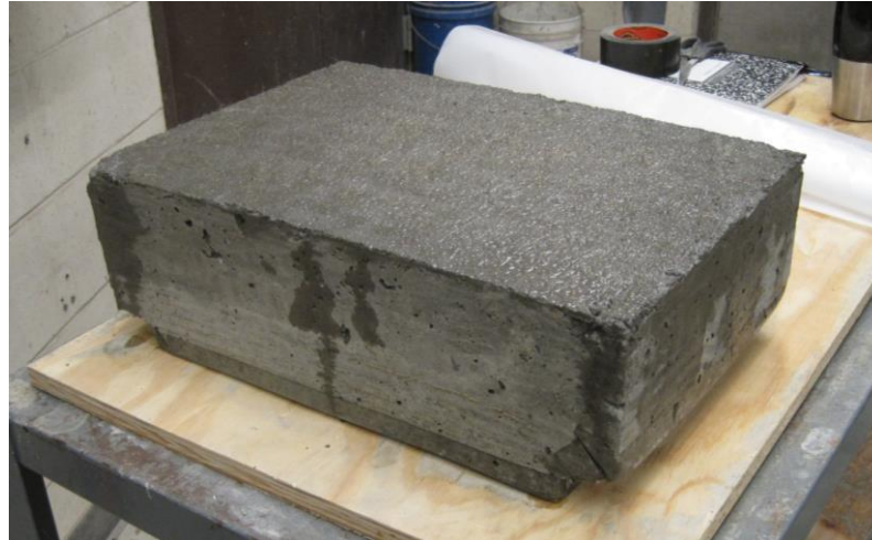
Figure 4: Slab after wet curing
