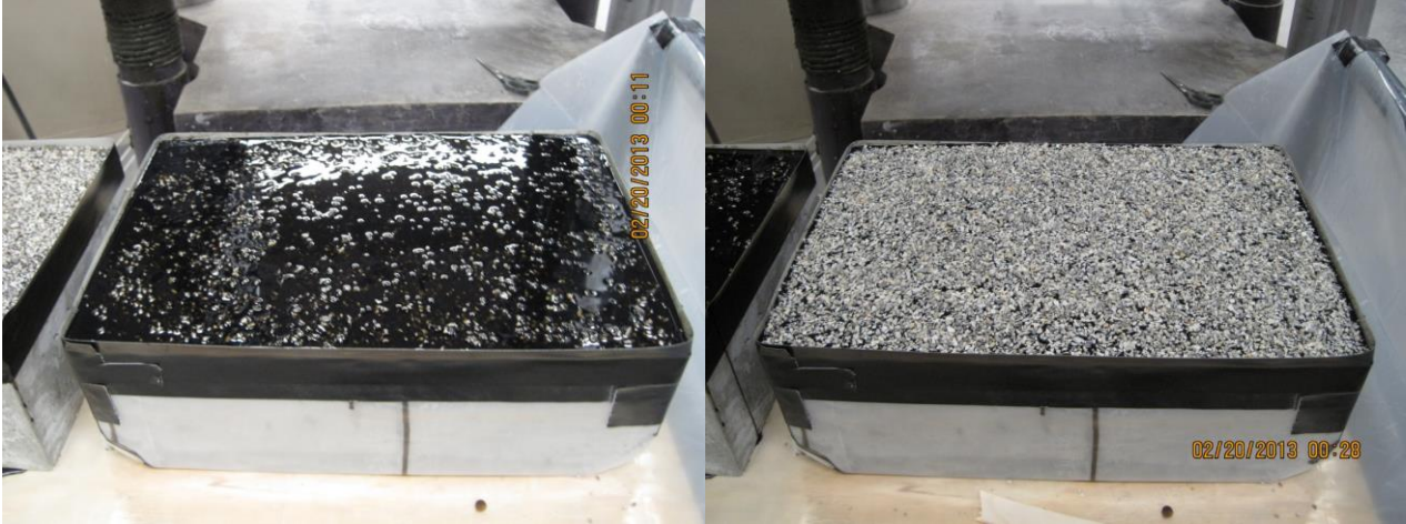
Figure 21: Placement of course 2 of epoxy (left) and aggregate (right)
