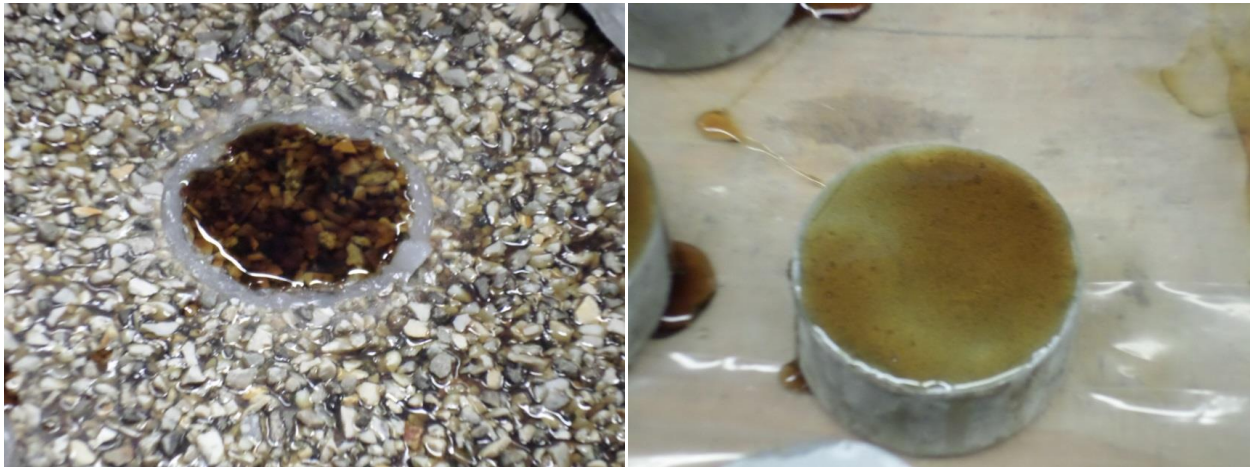
Figure 24: Application of adhesive epoxy to mount the aluminum caps
