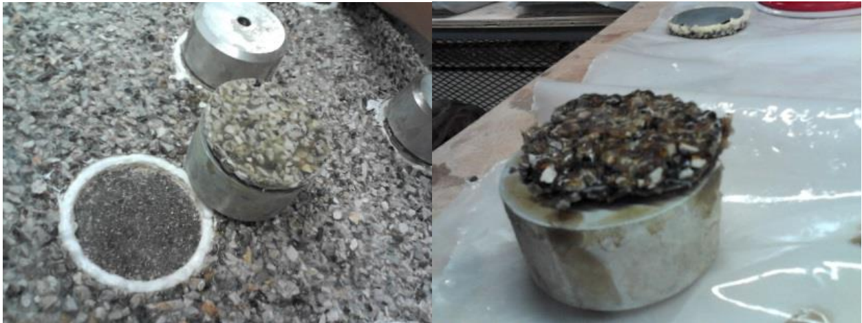
Figure 31: Failure type 3 (left) and failure type 4 (right)
