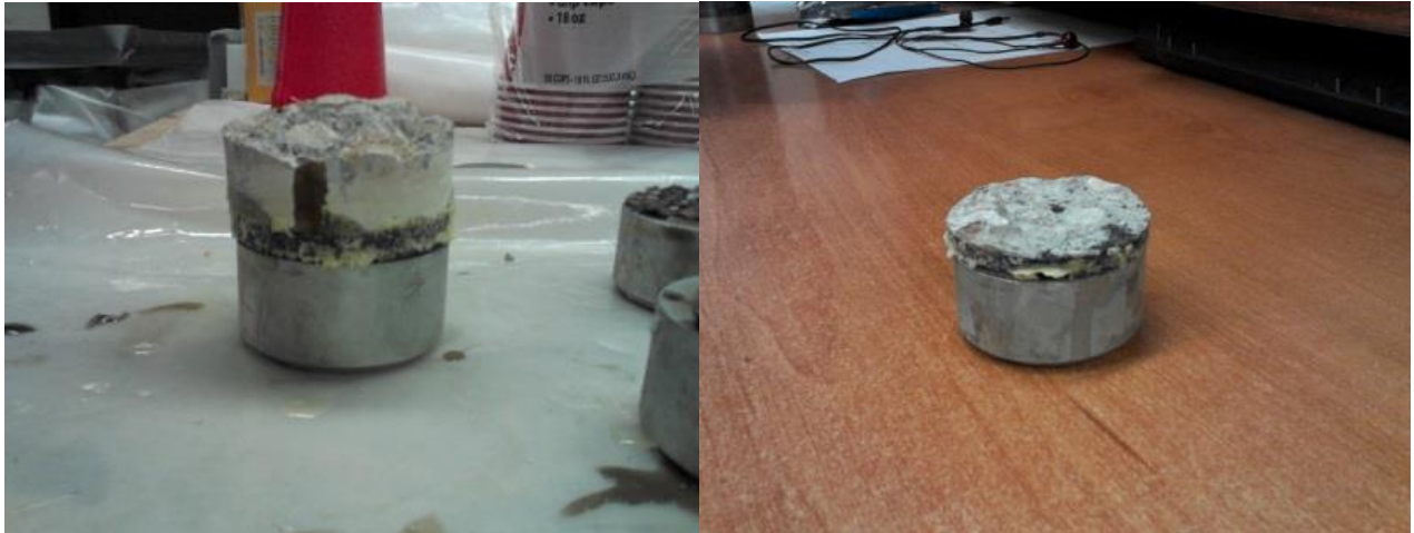
Figure 30: Failure type 1 (left) and failure type 2 (right)
