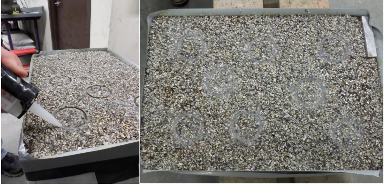
Figure 23: Placement of silicone caulk to seal the cores
