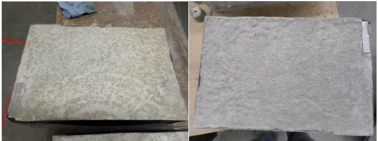
Figure 16: Before (left) and after (right) sand blasting a slab.
