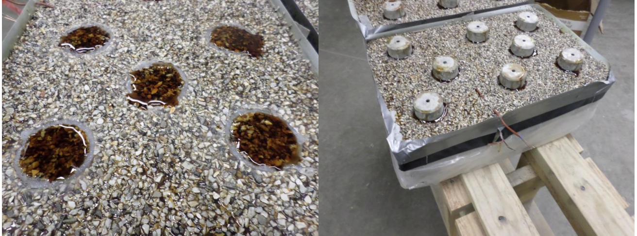
Figure 25: Slabs before and after placing pull-off caps.
