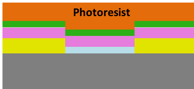
Figure A.9 PR spin coating. The thickness of PR is 0.7 μm with a recipe of P20 as the primer and 955-0.7 at the PR. The spin rate was 4000rpm for 45 sec.
