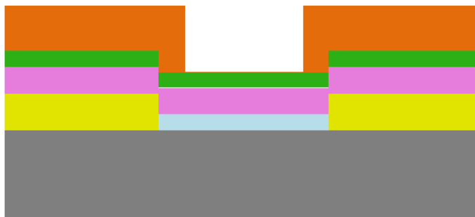
Figure A.11 Develop the pattern in CD-26 for 1 min. The quality of the photolithography was monitor under the microscope and the thickness of PR was measured by surface Profilometer.
