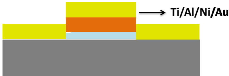
Figure A.5 Metal deposition to form Ohmic contact. Metal stack of Ti/Al/Ni/Au was evaporated in order by electron beam evaporation. The thickness of each layer is 25/20/40/50 nm. The first Ti layer reacts with N in GaN forming TiN which has low band offset with GaN. Meanwhile the N vacancy increase the conductivity of GaN. Al and Ni prevent the diffusion of Ti and Au respectively. Also, 40 nm of Ni provide better adhesion for Au layer
