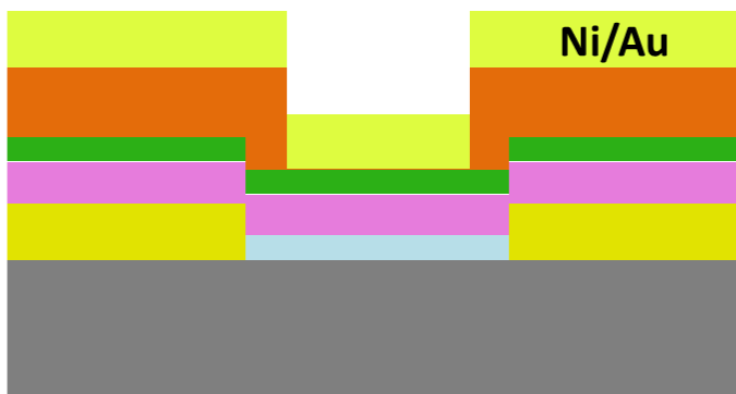
Figure A.12 Ni/Au (20/40 nm) was evaporated in order to form the gate contact.
