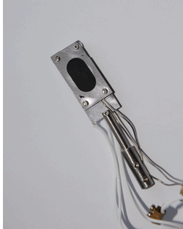
Figure 3.1 Sample holder-heater. The white color cables are used to provide the power for the heater, which consists of a plate of Ta. The shiny wires beneath the Ta frame are connected to the thermocouple. The black material in the middle of the frame is the sample (bucky paper) of DWNTs.
