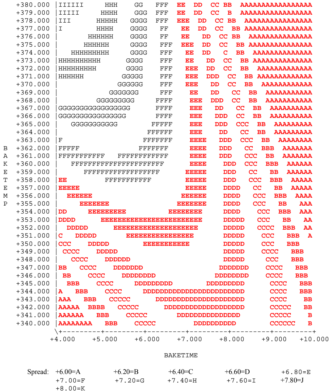
Figure 21. Effect of baking time and temperature on spread of blue corn cookies made in impingement oven
