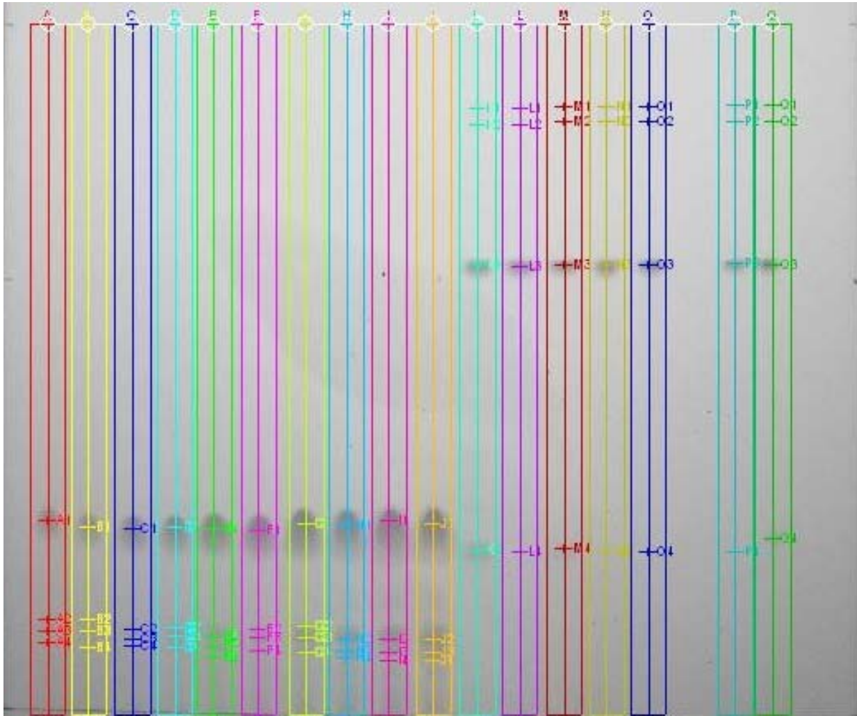
Figure 3.5 Sample TLC plate analyzed with Doc-It software
