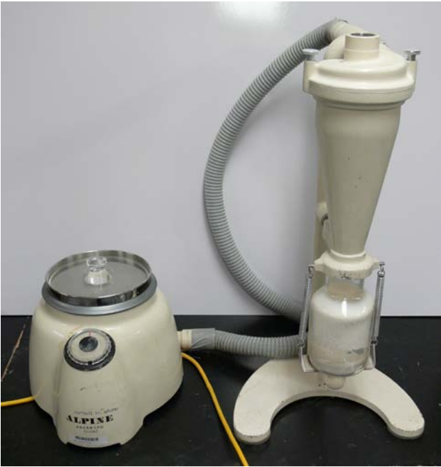
Figure 2.2 Alpine Air Jet Sieve
