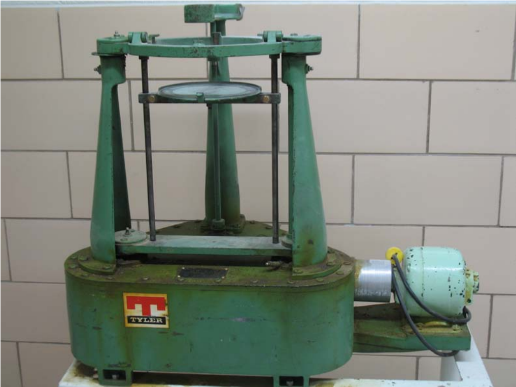
Figure 2.1 Ro-Tap Sieve Shaker
