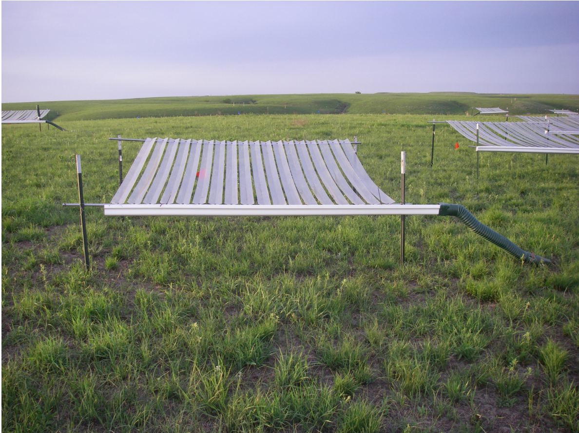
Figure 4.1: A 2.4 \times 2.4 m rainfall interception shelter, with shingles spaced to cover 80% of the total shelter area. Picture taken 26 April 2012 by B. VanderWeide.
