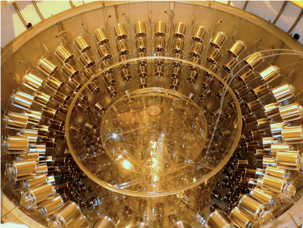
Figure 2.6: Various detector volumes in the Double Chooz main detector [43].
