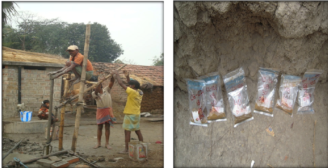
Figure 6: Local hand driven percussion drilling method (left); Sediments preserved inside in O 2 -impermeable Remel® bag with an O 2 absorber pouch inside. Flushed with N 2 gas and sealed (right)
