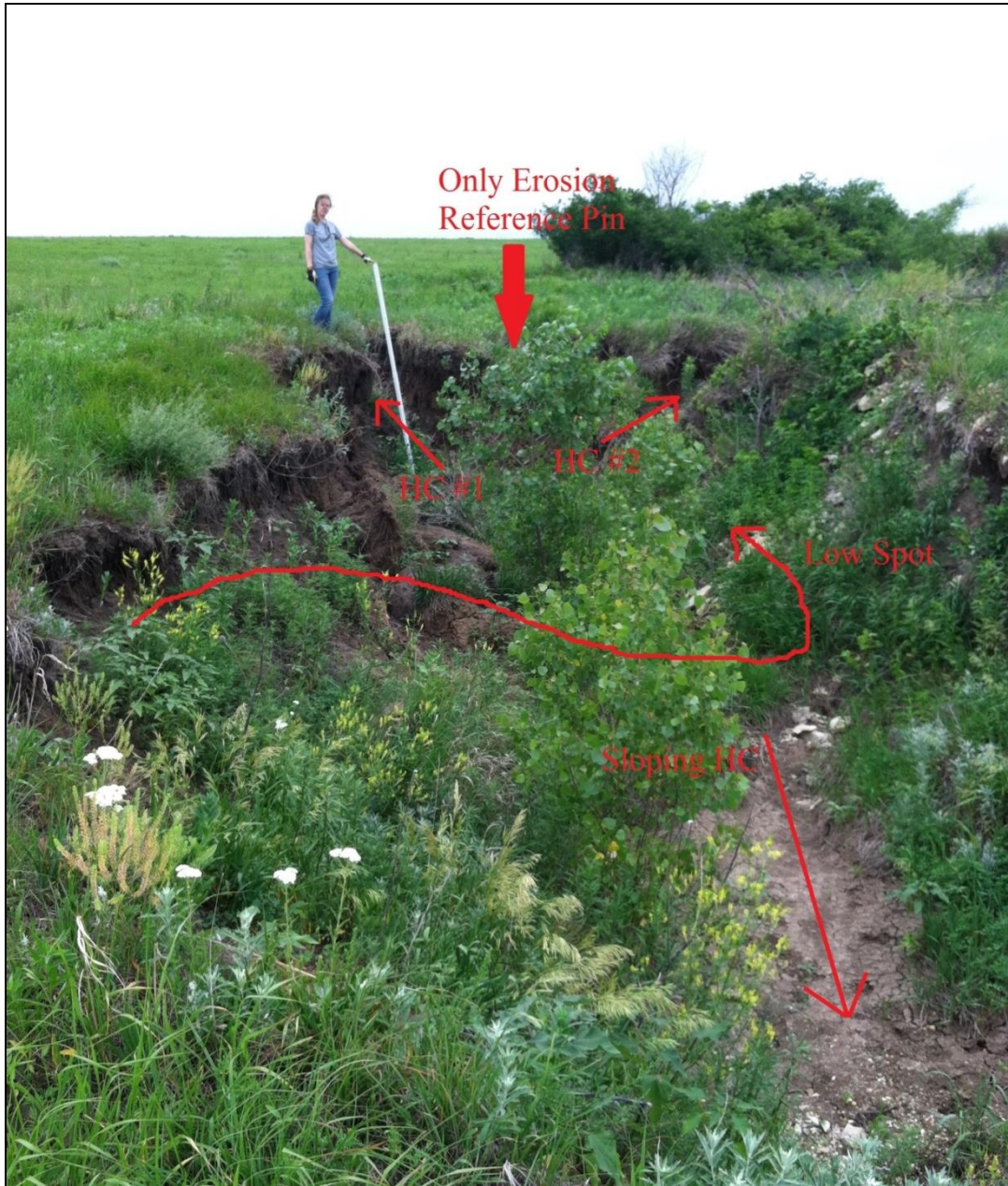
Figure 4.2. Unpredictable gully network (gully numbers 11 and 12, located in Training Area 95) with multiple headcuts, erosion features, and only one identifiable erosion reference pin
