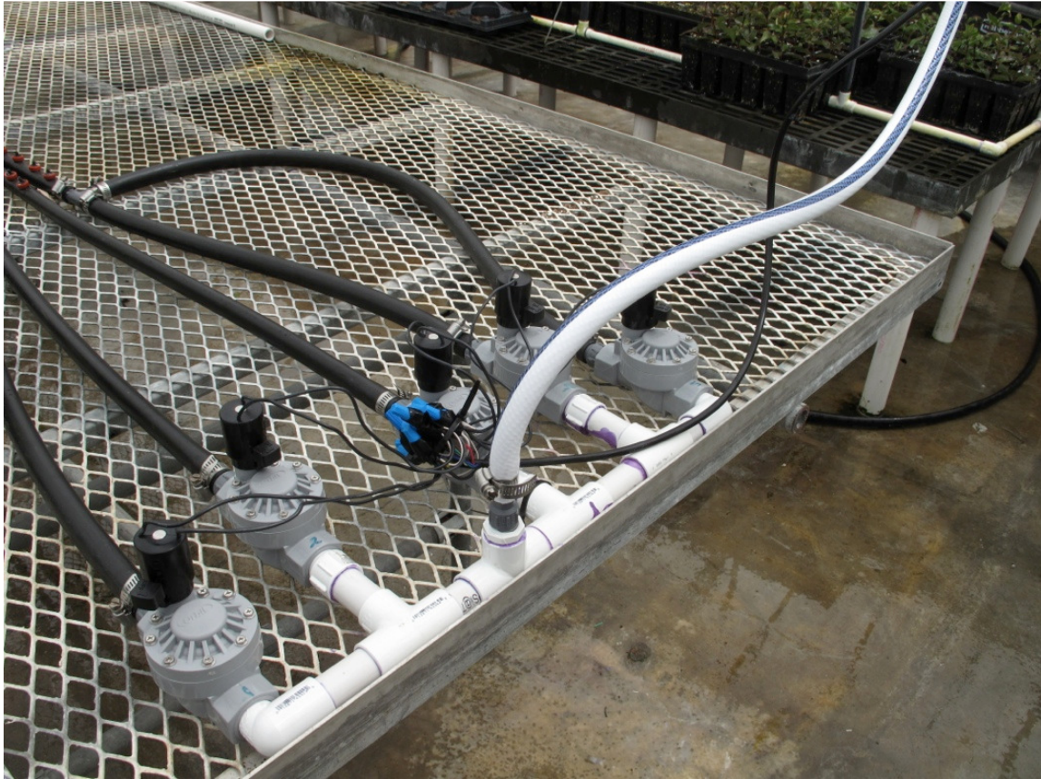
Figure 3.2 Irrigation setup including PVC manifold and solenoids used for cyclic irrigation alternative substrate study (sedum).
