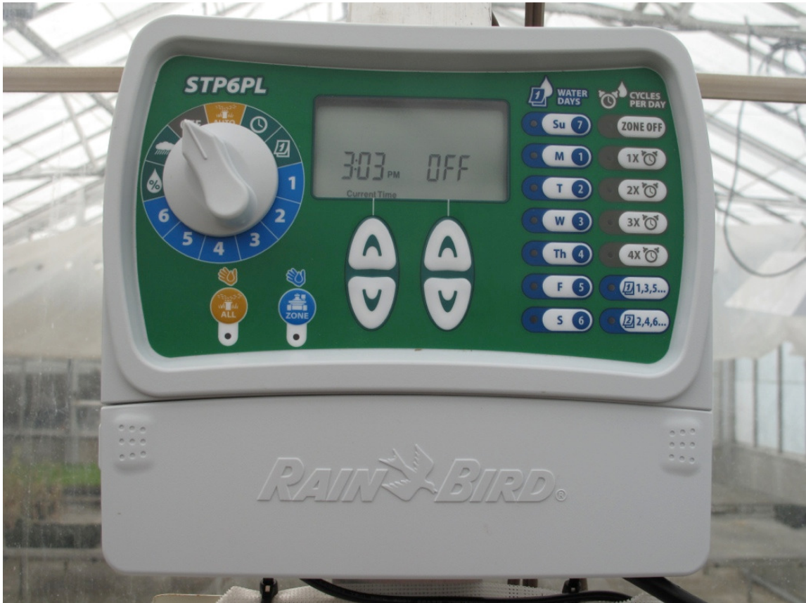
Figure 3.1 Rain Bird irrigation controller used for first cyclic irrigation in alternative substrate study (sedum).
