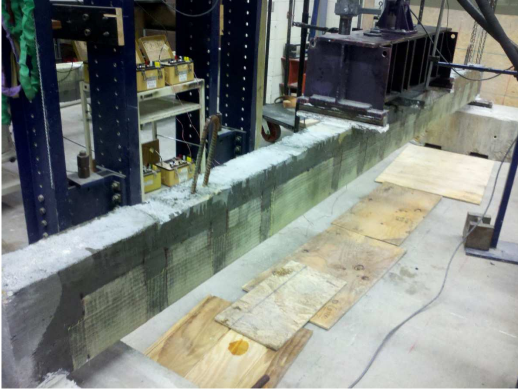
Figure 37: Setup of Beam R3 before Testing
