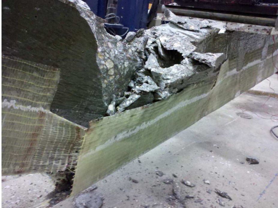
Figure 44: Crushed Concrete and Debonded U-Wrap on Specimen R4
