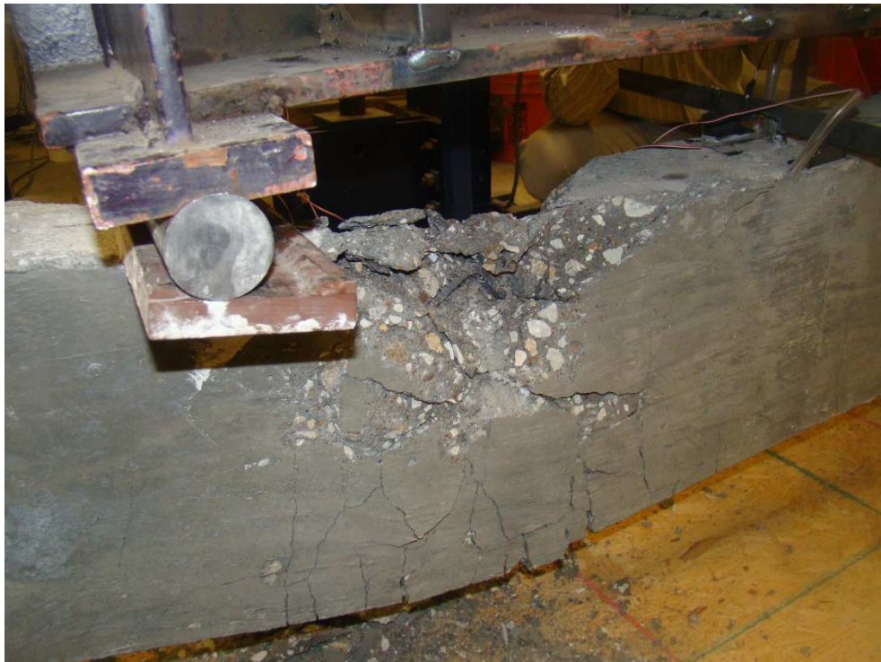
Figure 32: Concrete Crushing of Control Beam
