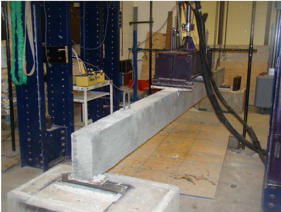
Figure 30: Setup of Beam R1 before testing
