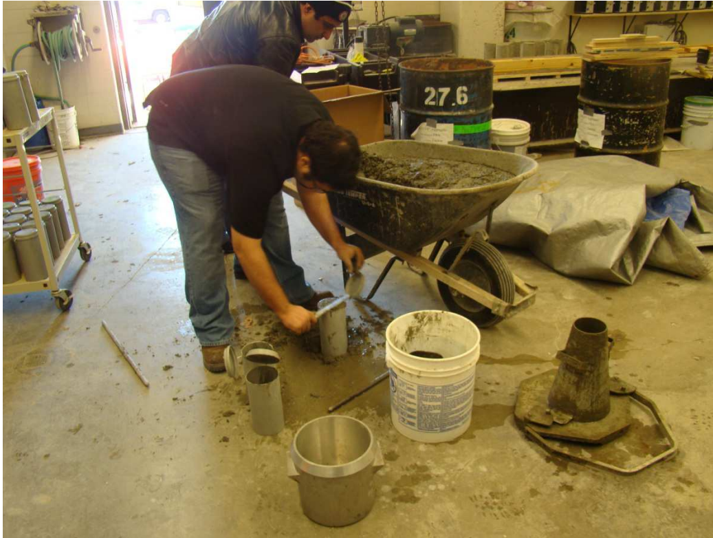
Figure 11: Casting of Concrete Cylinders
