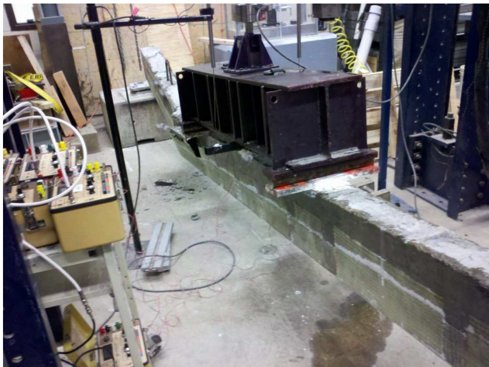
Figure 43: Failure of Beam Specimen R4
