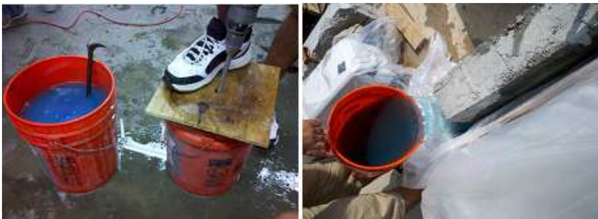
Figure 29: Mixing 25% by-weight saline Solution (left) and Applying Solution to Specimen R4 (right)
