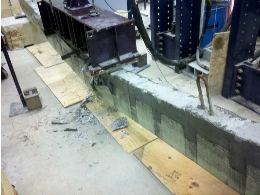
Figure 34: Full Length NSM Beam at Failure
