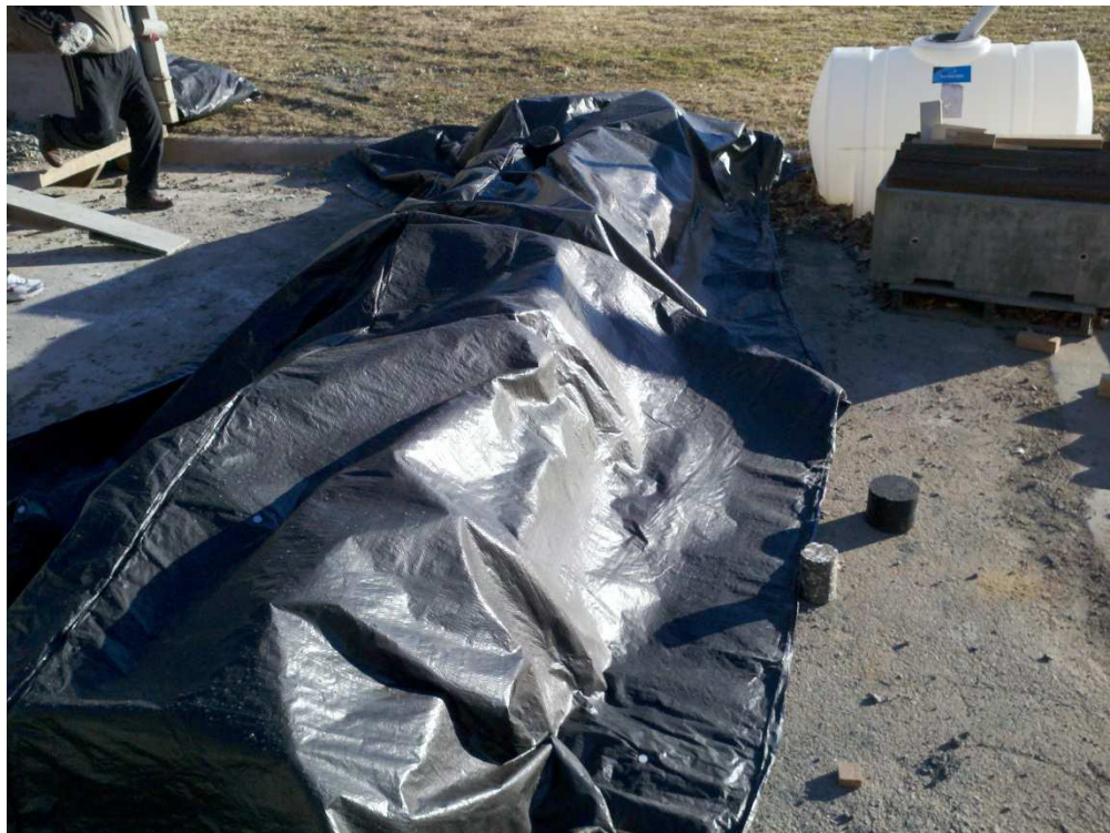
Figure 12: Covering Specimens with Concrete Blanket
