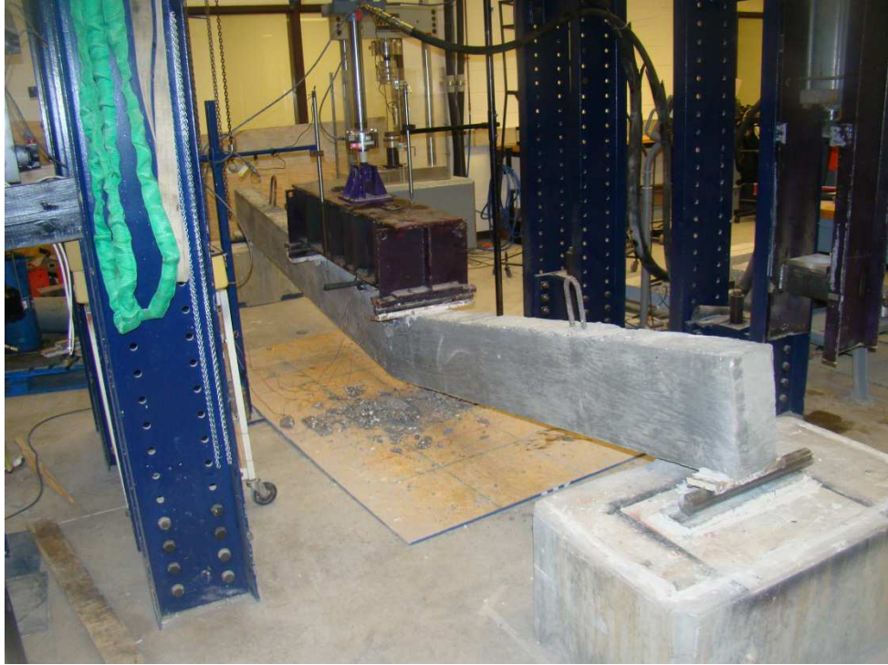
Figure 31: Control Beam at Failure
