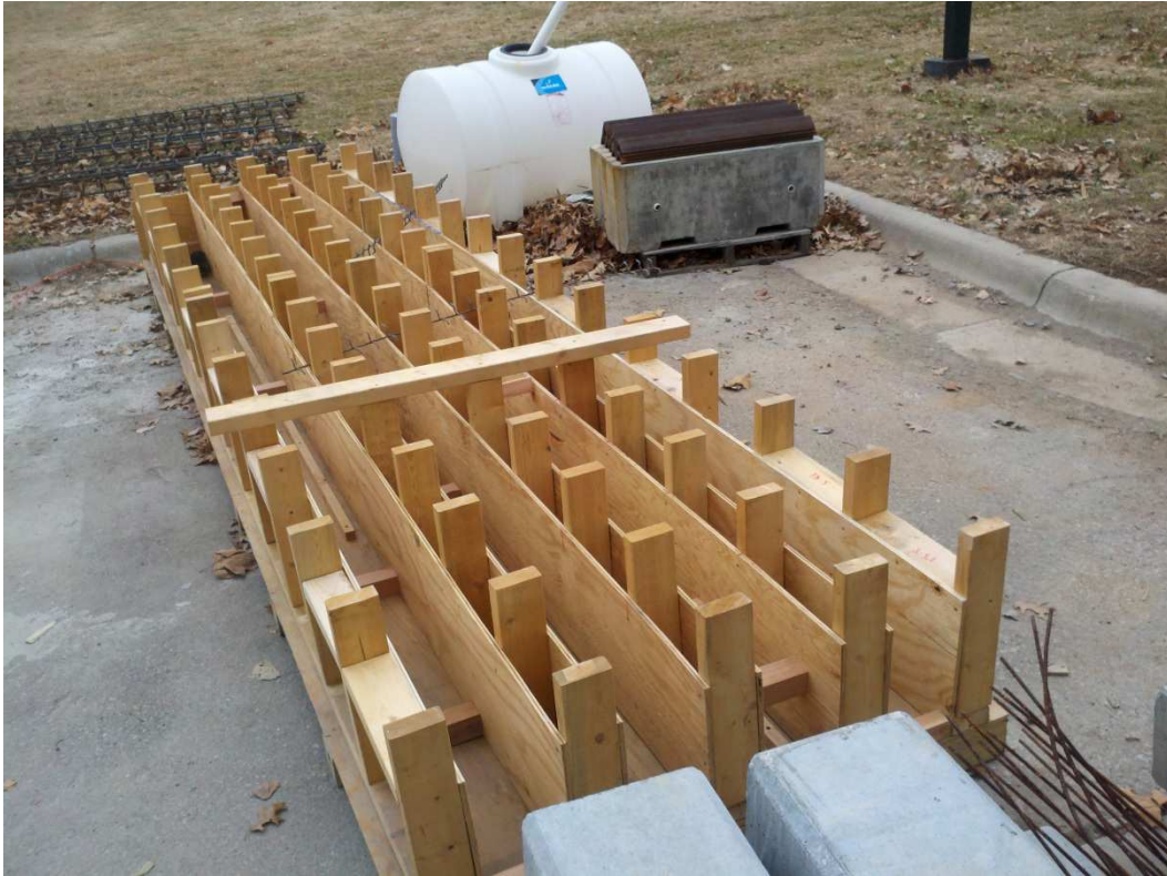
Figure 5: Formwork for the Beam Specimens
