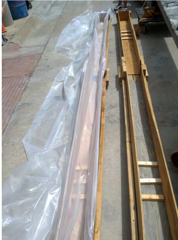
Figure 28: Formwork and Plastic Lining for the Corrosion Test
