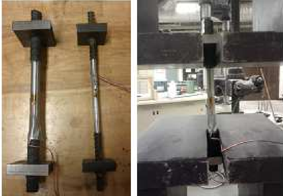
Figure 25: Bars with Strain Gages attached (left) and Testing Bar in Hydraulic Frame (right)
