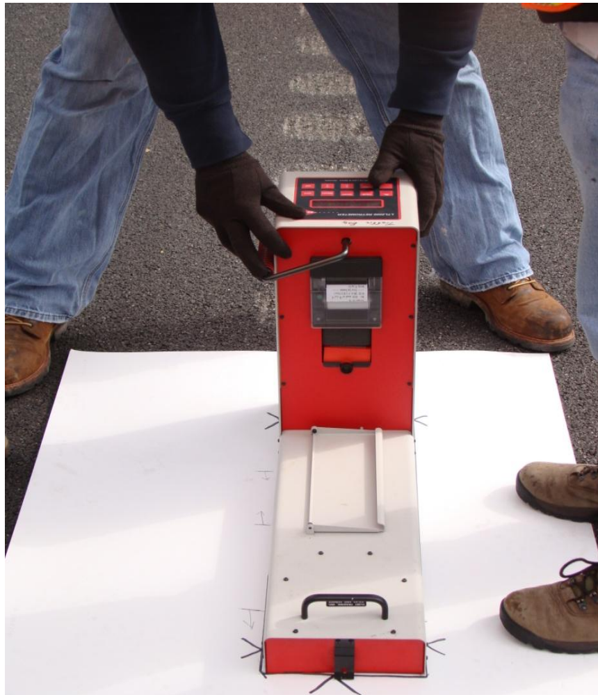
Figure 5.5 Retroreflectivity measurement on CLRS using Reflectometer LTL 2000 kept on hardboard.
