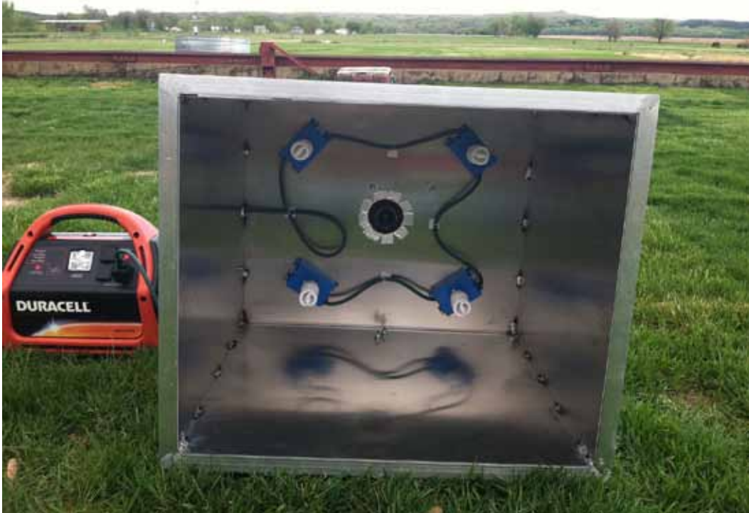
Figure 1. Internal view of the light box showing the wiring and light bulb placement.
