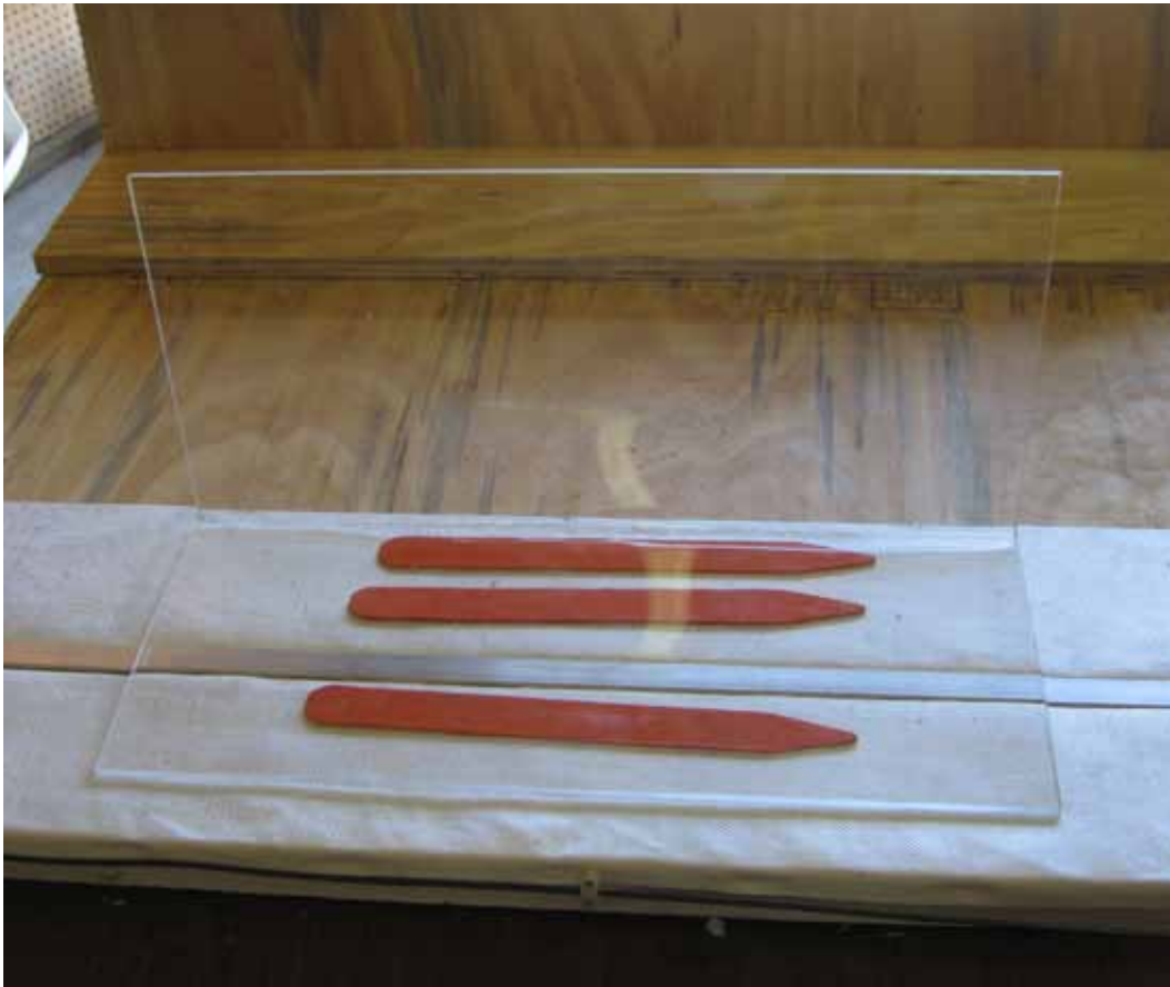
Figure 1. A custom-made acrylic bender that uses a strip heater makes acrylic pliable enough to bend.
