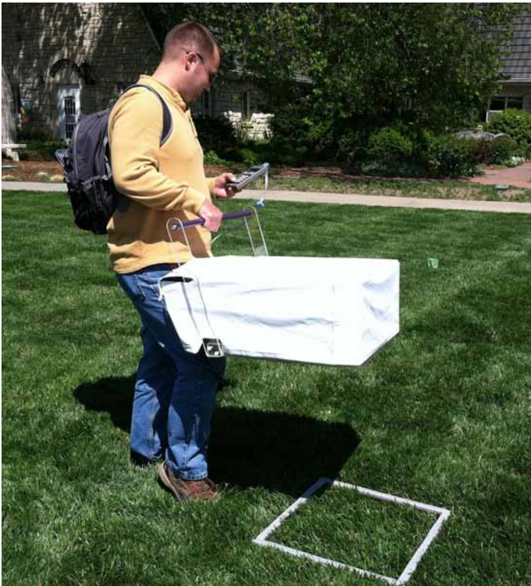
Figure 3. The new fabric cover facilitates dark measurements. The operator is wearing the backpack containing the data logger and battery.
