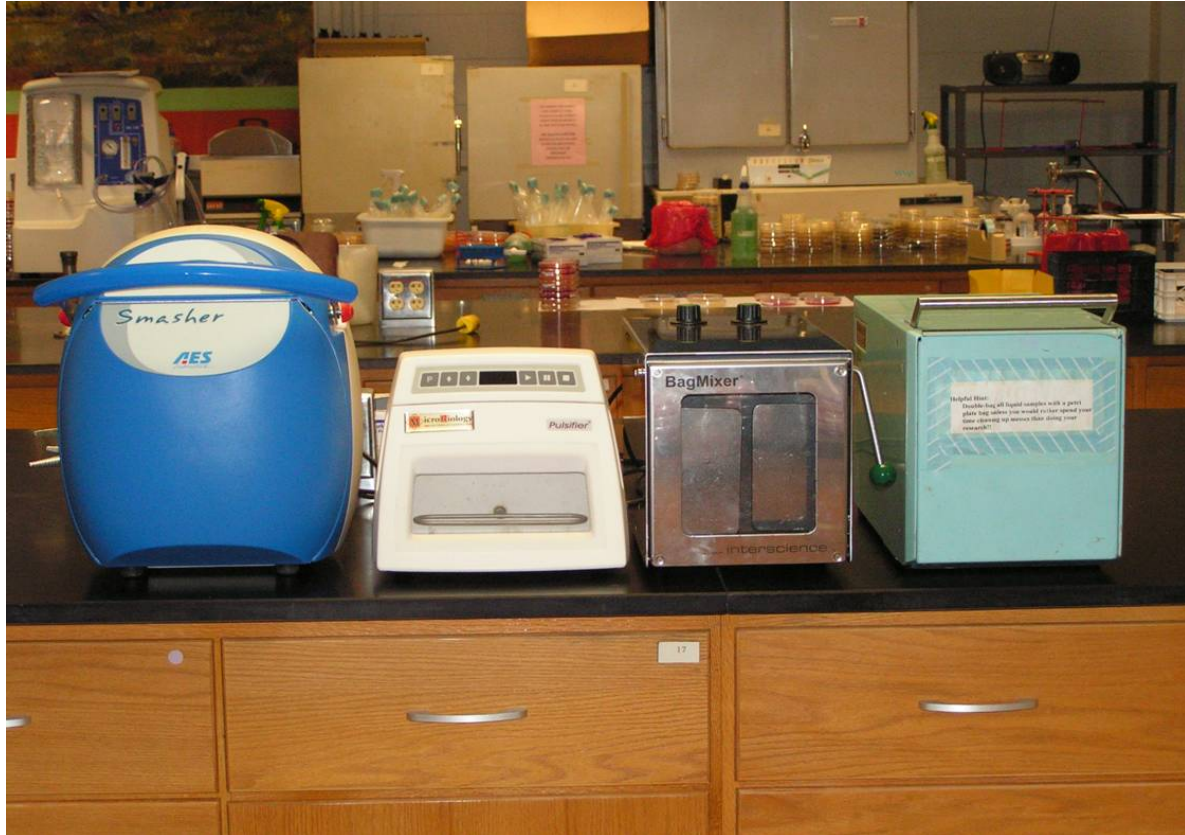
Figure 5 Instruments used in the experiment. From left to right, the Smasher® (AES-Chemunex, 1 Corporate Drive, Cranbury NJ), Pulsifier® (Microbiology International, 5111 Pegasus Court, Suite H, Frederick MD), Bagmixer® (Interscience, 301 Winter ST, Hanover MA), and Stomacher® (Seward Laboratory Systems Inc, 1648 Locust Avenue, Bohemia NY).
