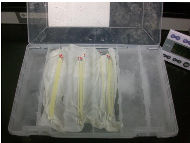
Figure 7.4 Ice block used to provide 0°C conditions.
