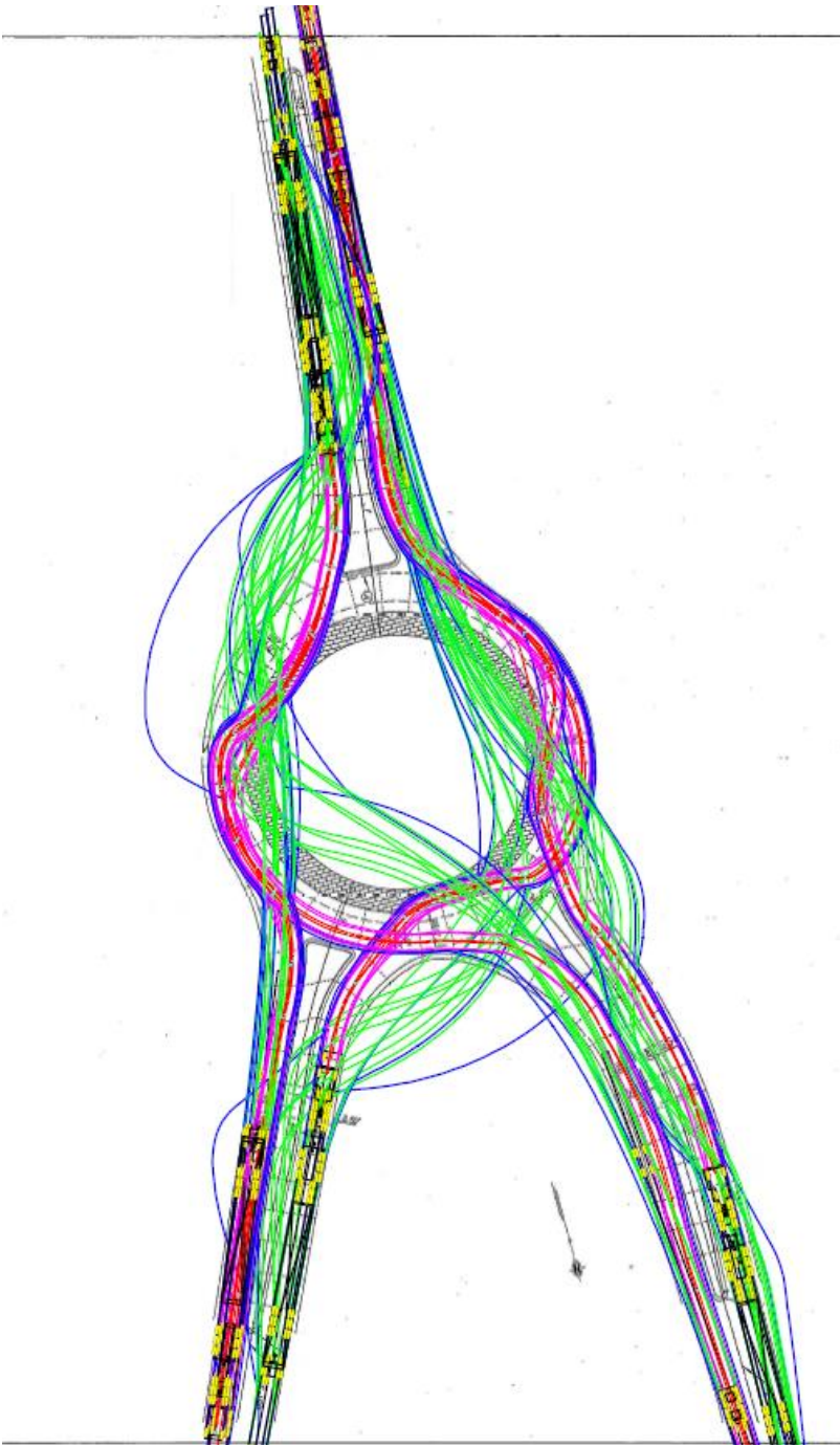
Figure 4.38: Garnett Roundabout Showing all Critical Vehicle Simulations for all Approaches
