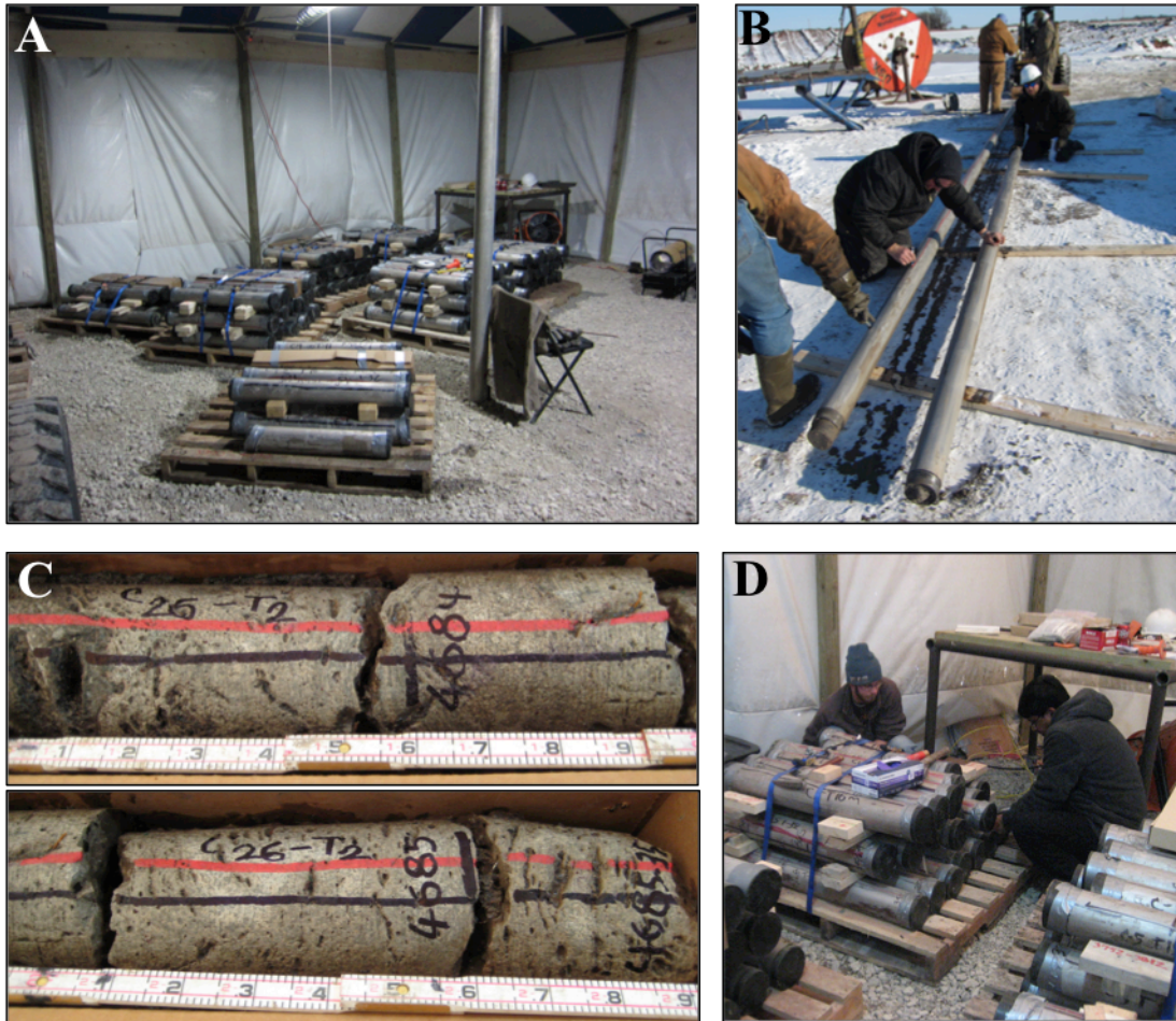
Figure 4-1. (A) Core sections stored on pallets in climate controlled tent awaiting transportation to Weatherford Laboratories in Houston, TX. (B) Marking the depth and orienting the 30` core sections before cutting into smaller sections. (C) Whole core sections without aluminum sleeves marked with depth and top-bottom orientation descriptions. (D) Collecting core chips from the end of 3` core sections.
