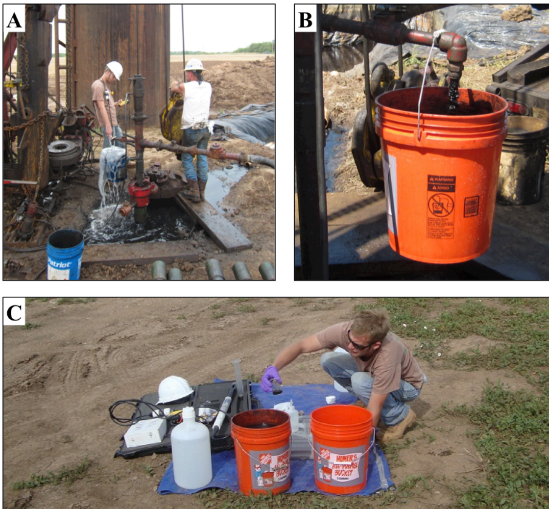
Figure 4-4. (A) Monitoring physical chemistry of swabbed water using HACH Hydrolab MS5 at KGS 1-32. (B) Black water produced during the first minute of each swab test. (C) Conducting field analyses of swabbed water.
